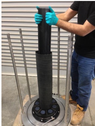
e. Seating the pedestal base (with porous stone part and inner membrane) on the base of the chamber and securing with bolts
