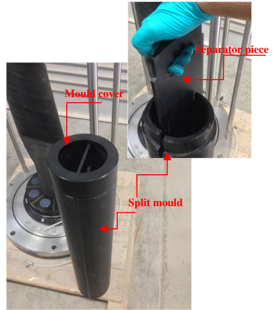
f. Inner split mould assembly
