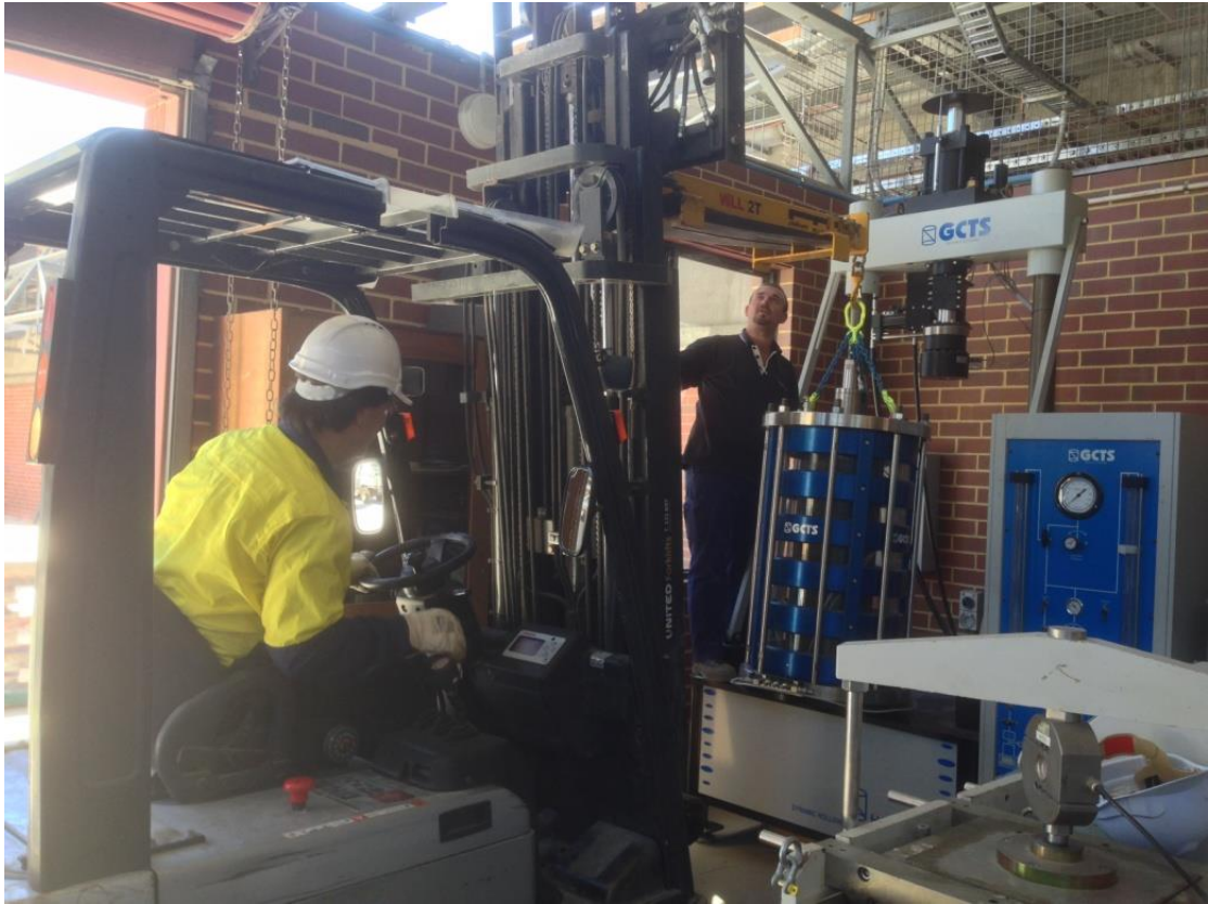
t. Using a forklift to lift and set the sample up in the hollow cylinder apparatus
