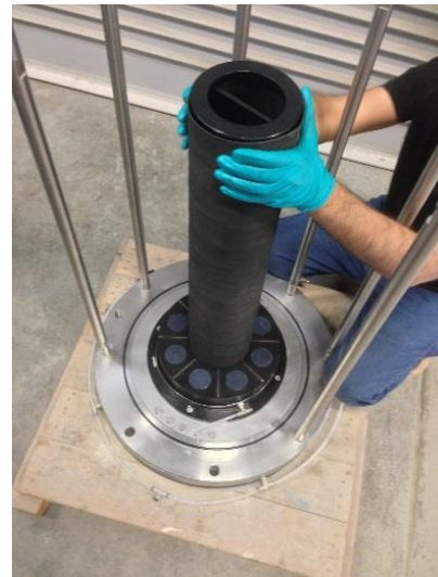
g. Erecting the inner split mould assembly inside the inner membrane
