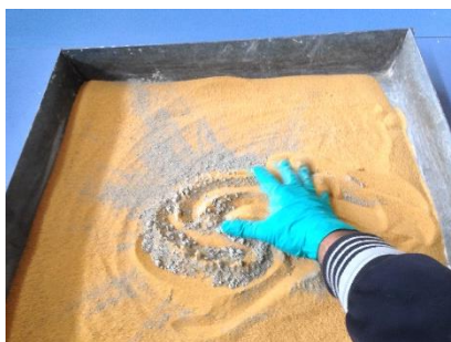
(d) Sand-cement is thoroughly mixed by hand
