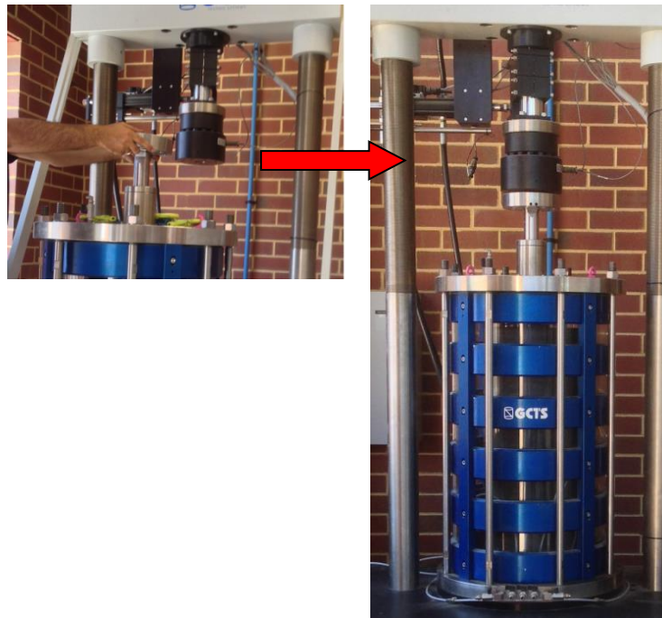
t. Using a forklift to lift and set the sample up in the hollow cylinder apparatus
