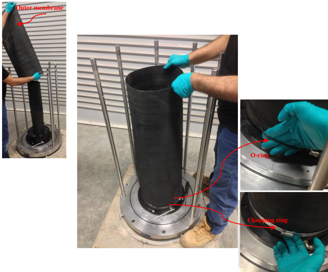
h. Fastening the outer membrane outside the pedestal using a clamping ring
