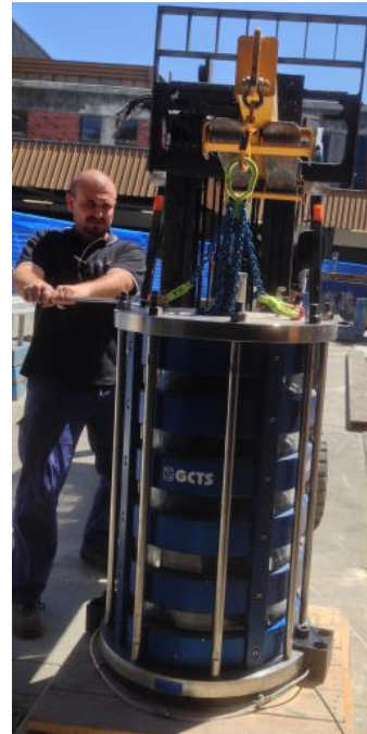
s. Tightening the cell chamber on the prepared sample
