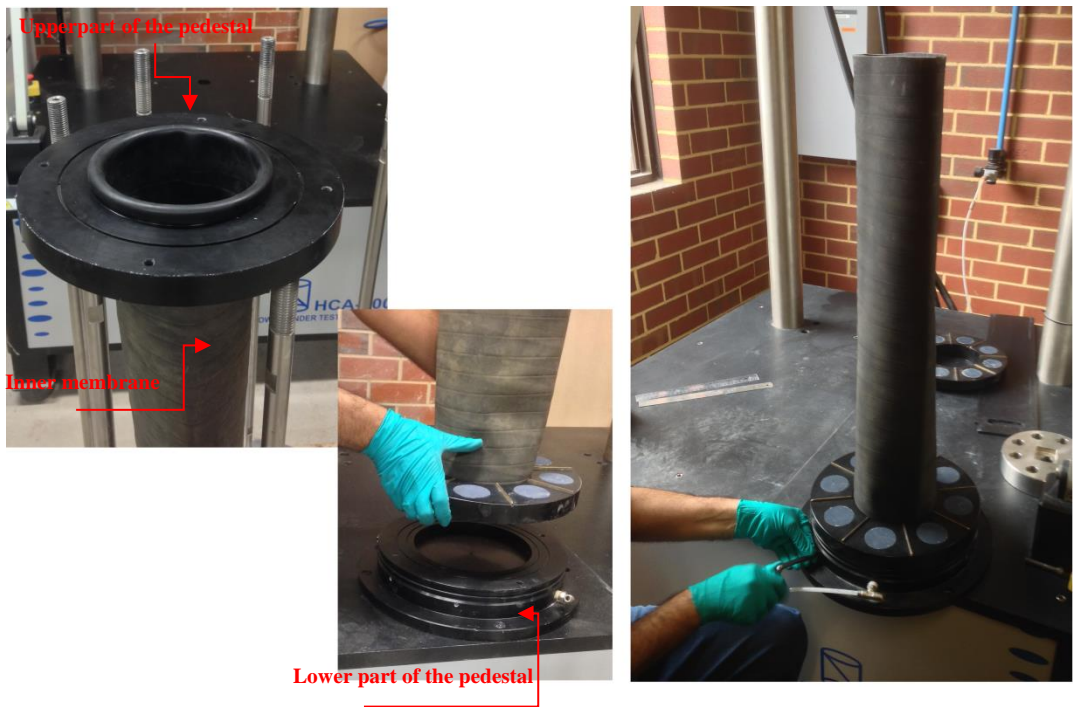
d. Fixing the inner membrane inside the porous stone compartment and fastening them on the base of the pedestal
