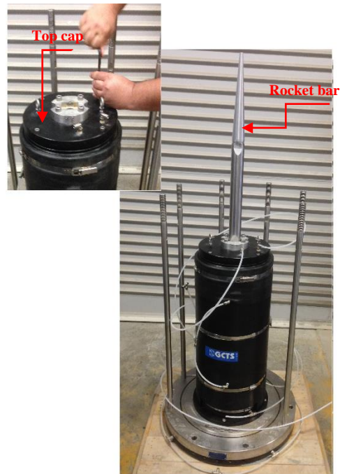
m. Seating the top porous stone gently on the top of the specimen
