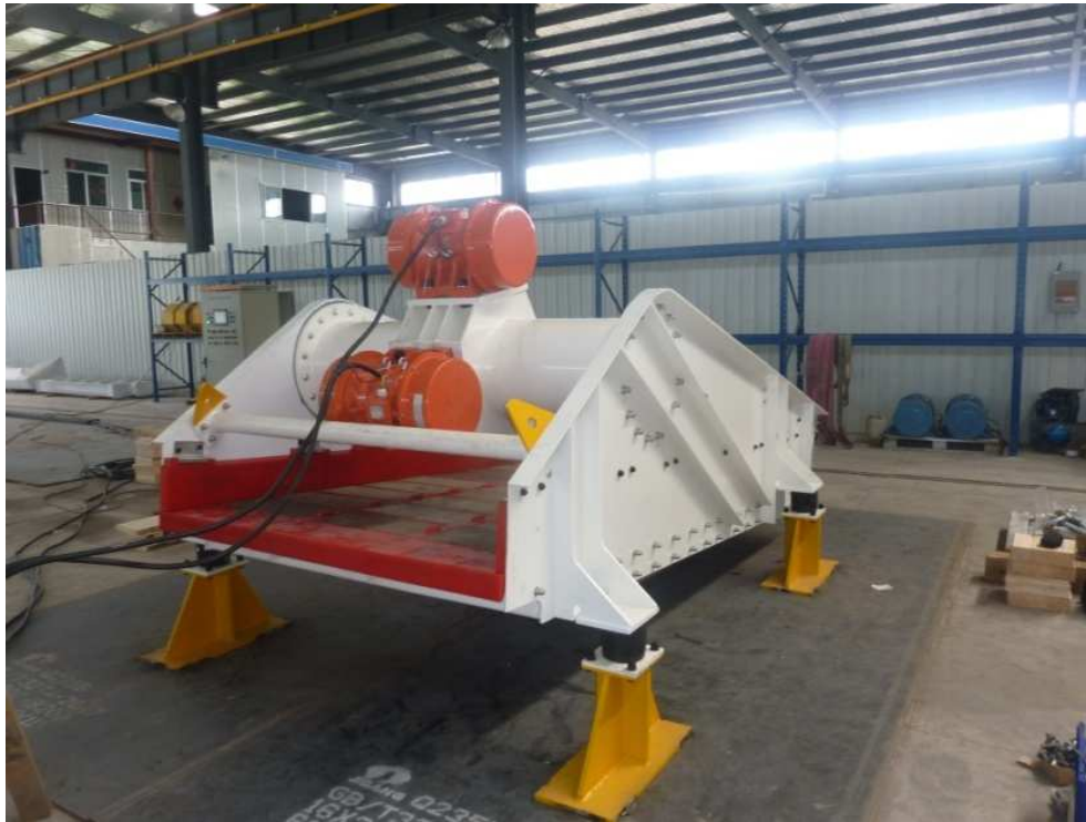
Figure 3.11 Vibrating screen with two electric vibrators operating in counter-directions
