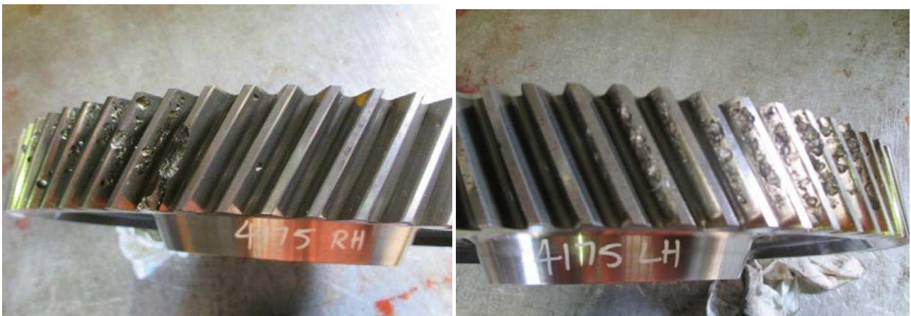
Figure 7.5 Pitting of the gears
