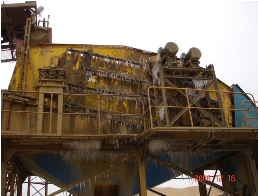
Figure 3.8 Vibrating screen with two unbalanced shafts driven by two separate electric motors
