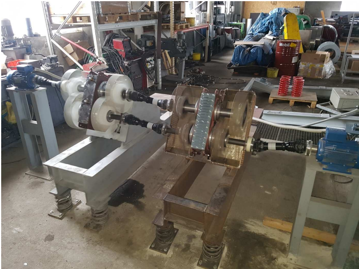
Figure 7.24 Two testing rigs with gearless exciters driven with two electric motors (Goster P/L).
