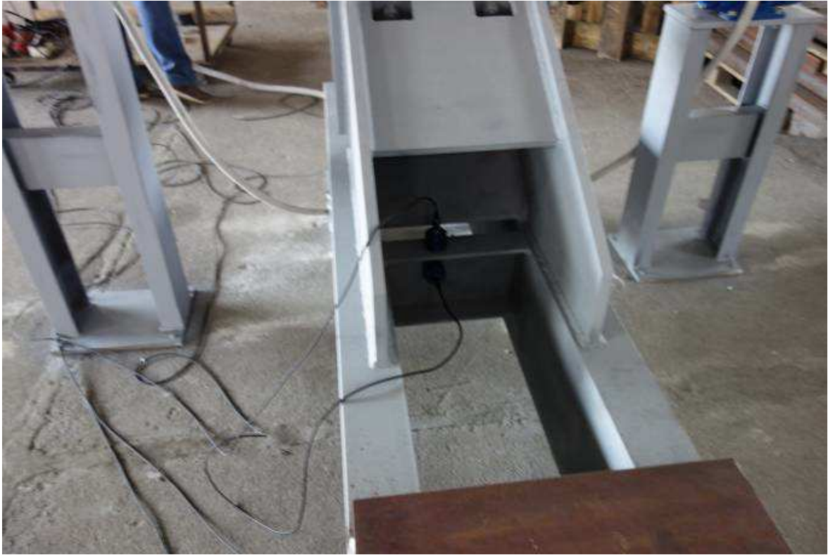
Figure 7.12 Accelerometers in the middle on the gearless exciter testing rig
