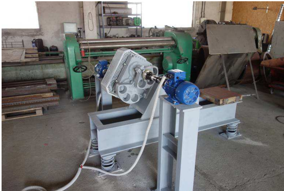
Figure 7.9 Gearless exciter on the test stand
