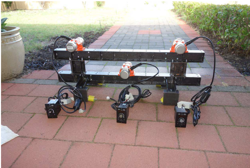
Figure 4.3 Initial setup of the testing rig with original counterweights and urethane springs
