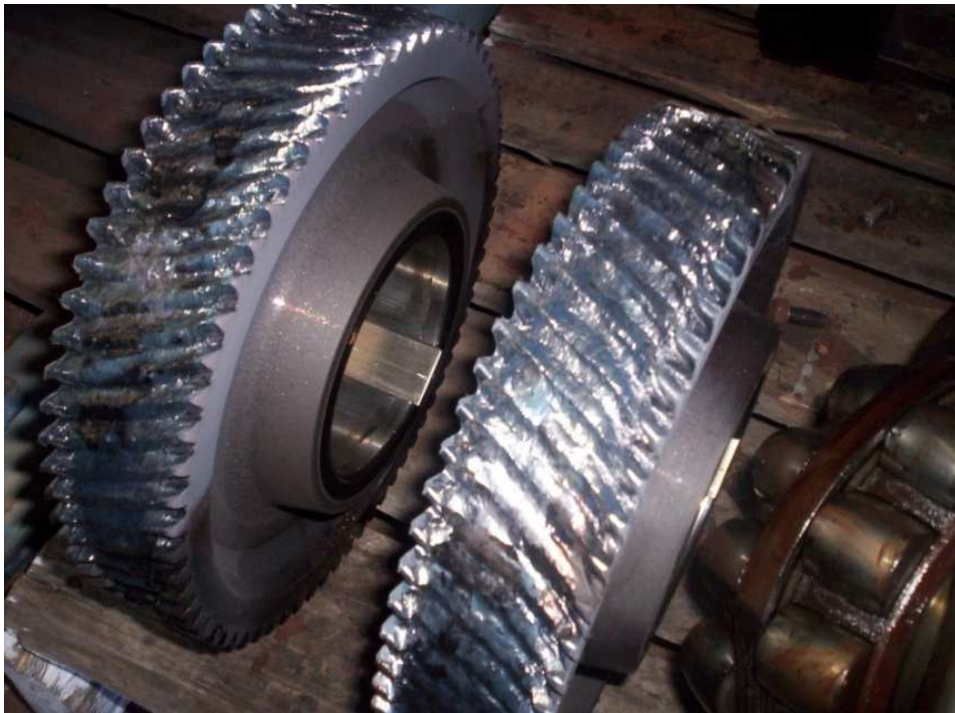
Figure 7.8 Damaged gears as a result of seized bearings.
