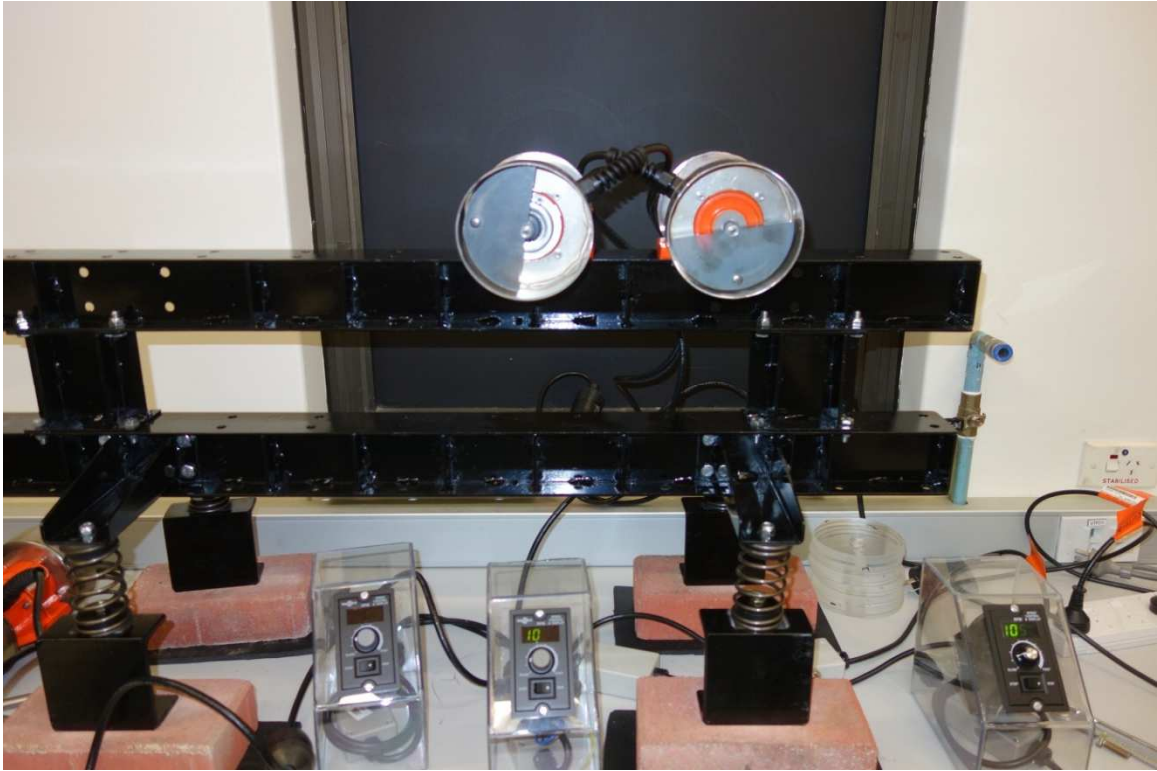
Figure 10.4 Two vibrators operating in opposite directions
