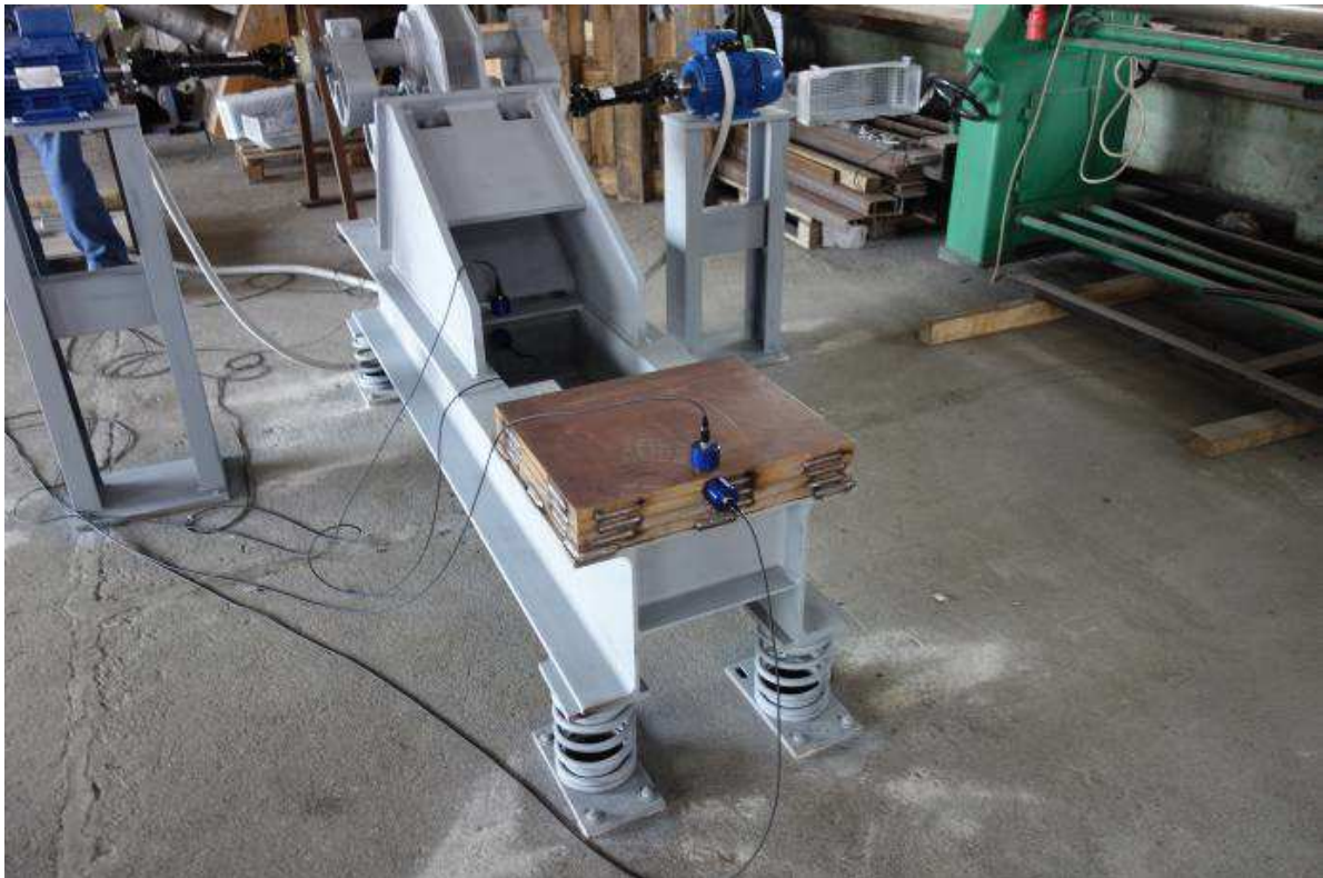
Figure 7.13 Accelerometers at the back location on the gearless exciter testing rig
