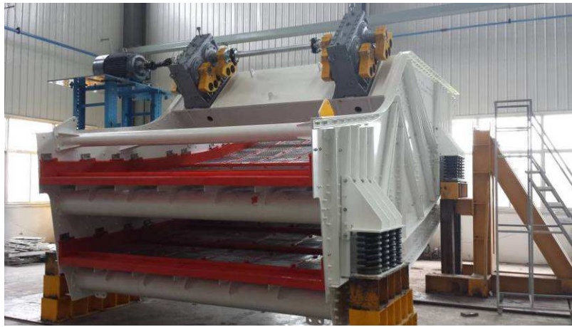
Figure 7.2 Example of a vibrating screen with 2 exciters connected with a single shaft
