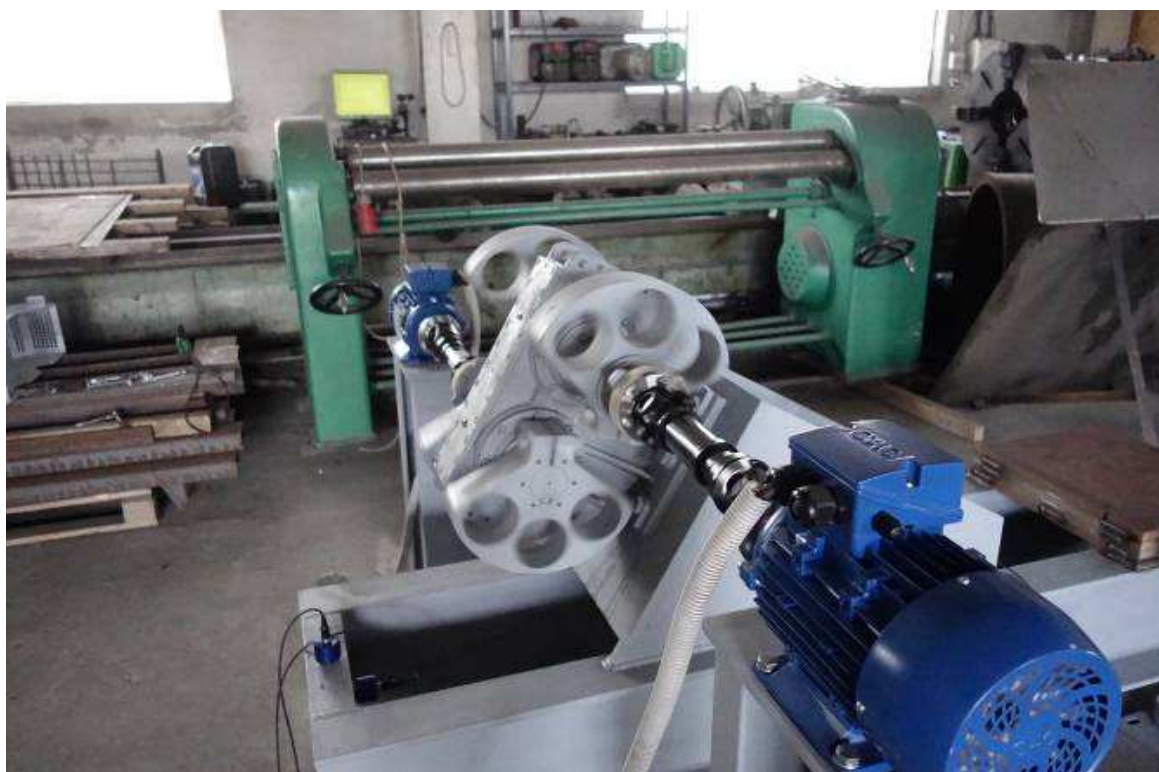
Figure 7.11 Front end accelerometers location on the gearless exciter testing rig
