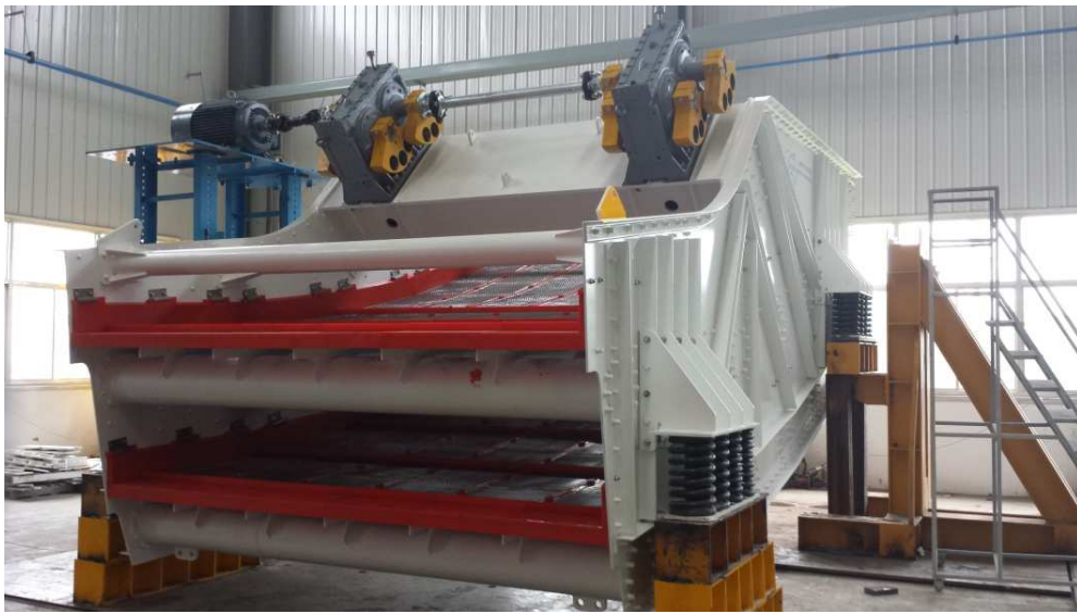
Figure 3.10 Typical vibrating screen with two geared box type exciters
