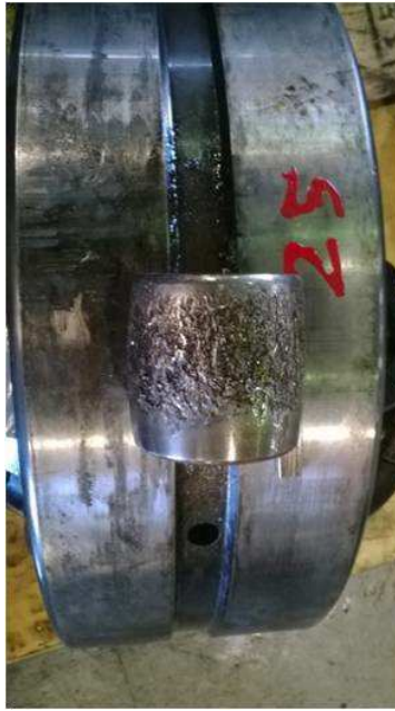
Figure 7.6 Present damage to bearing caused by metal particles in the lubricating oil
