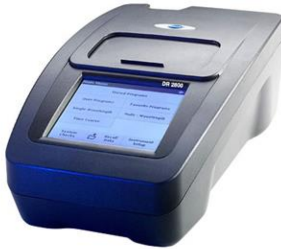
Figure 3.8 HACH DR-2800 Spectrophotometer
