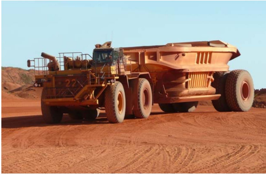
Figure 3.5: Cat bottom-dump type truck used to haul the extracted bauxite material. The capacity is 150 tonne (Erten, 2012)
