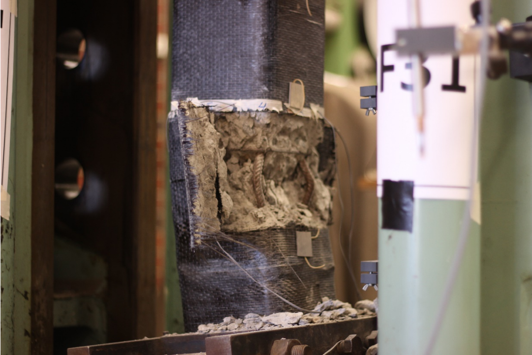
Figure 4.3.1-12 Concrete crushing and rebar buckling in compressive zone of CF31
