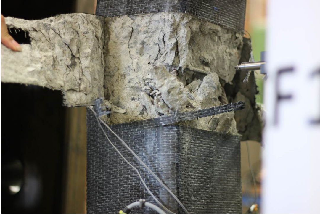
Figure 4.3.1-5 Concrete crushing in the compressive zone of CF11
