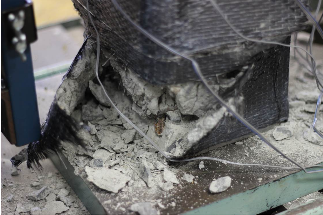
Figure 4.2.1-7 Concrete crushing and CFRP rupture at the bottom of specimen
