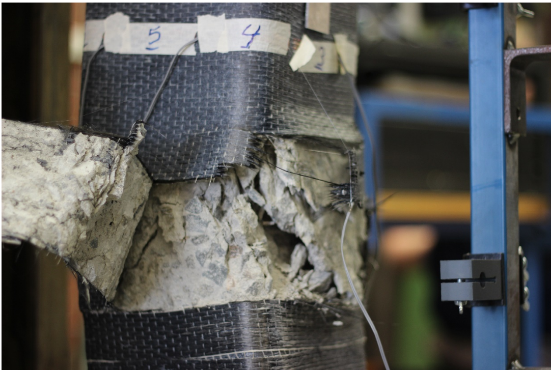
Figure 4.5.1-9 Concrete crushing and CFRP rupture in the compressive zone of CF23
