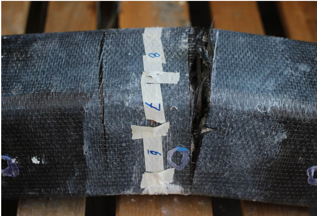
Figure 4.6.1-7 Flexural failure and longitudinal rebar rupture in CF2B
