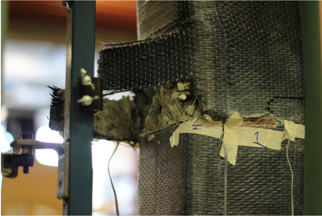
Figure 4.4.1-10 Concrete crushing and CFRP rupture in CF22
