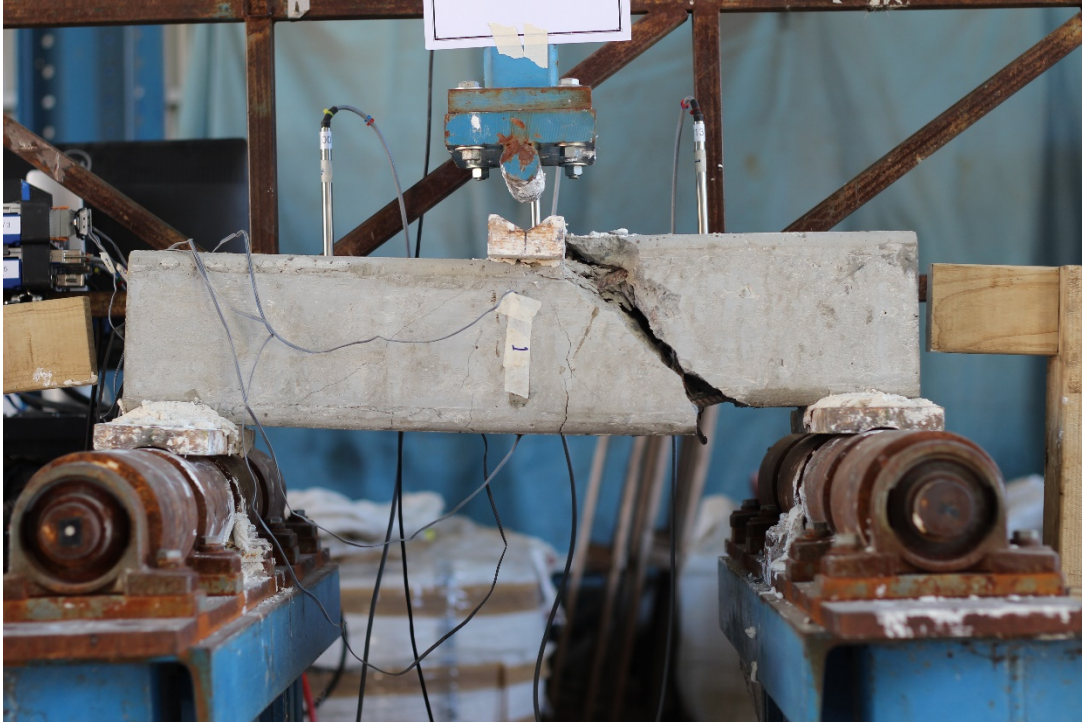
Figure 4.6.1-2 Propagation and localization of diagonal shear cracks in CRB
