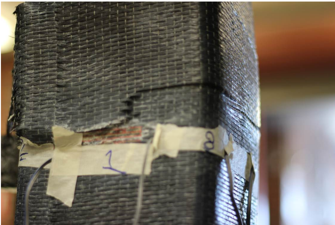
Figure 4.4.1-9 CFRP rupture and tearing in CF22
