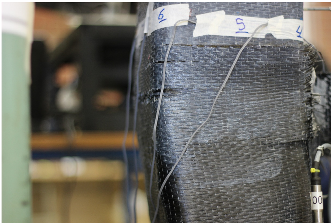
Figure 4.4.1-14 CFRP tearing in specimen CF32
