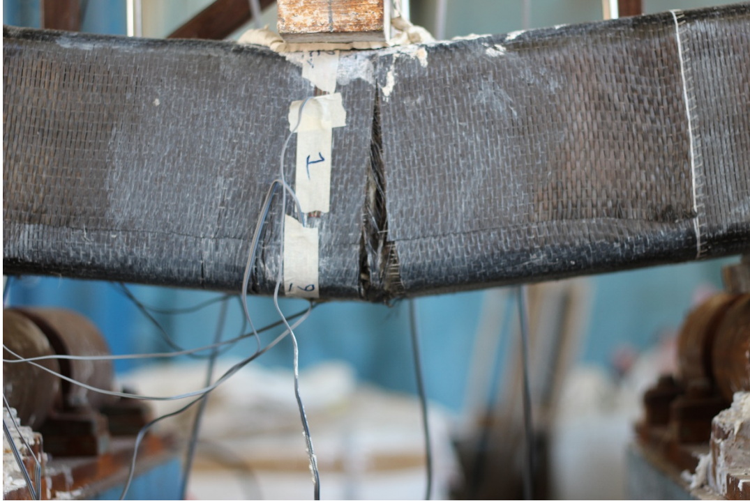
Figure 4.7-2 Direction of CFRP fabrics relative to the direction of beam axis
