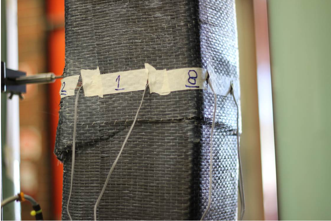
Figure 4.5.1-12 CFRP rupture and tearing in the tension zone of CF33
