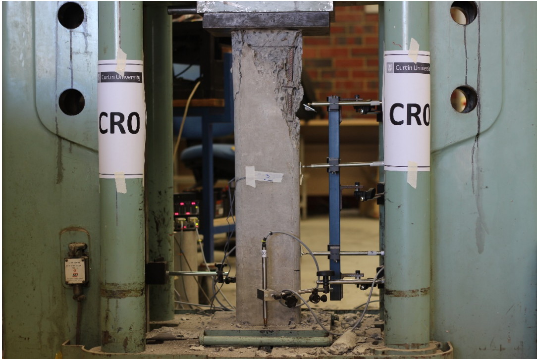
Figure 4.2.1-1 Overall view of CR0 failure
