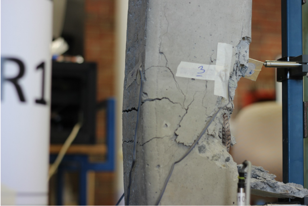
Figure 4.3.1-2 Concrete cracking in the tension zone of CR1
