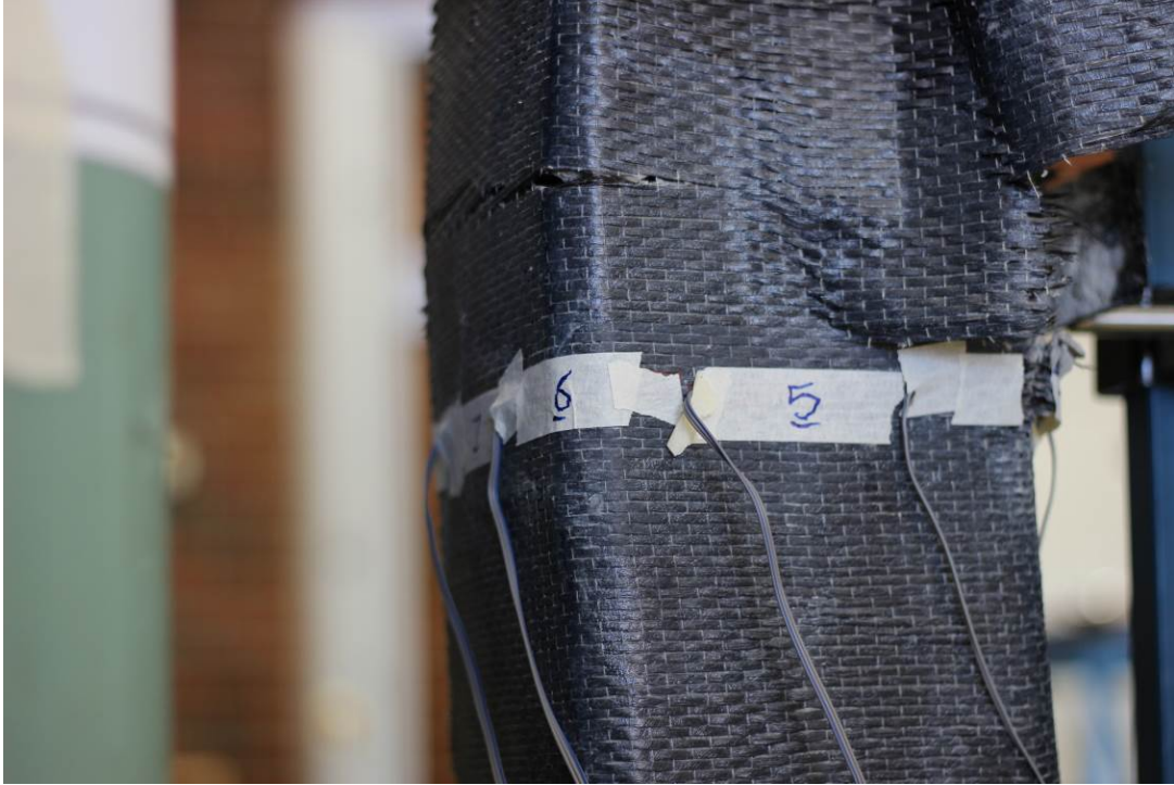
Figure 4.4.1-7 Torn CFRP in tension zone of CF12
