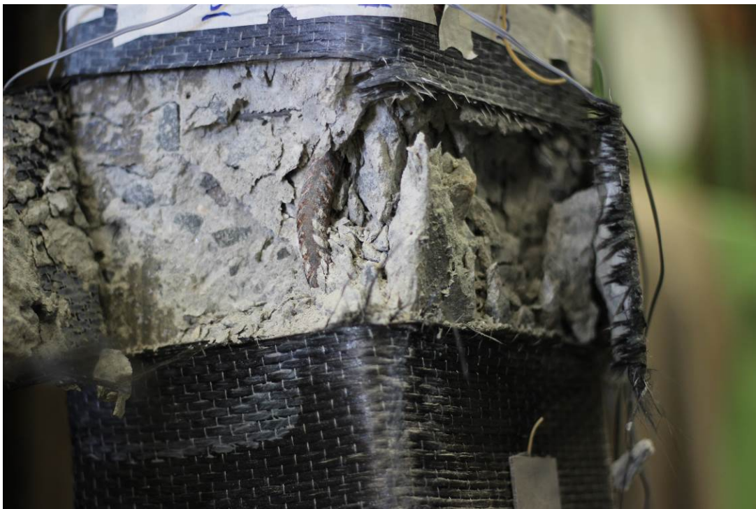
Figure 4.4.1-13 Concrete crushing and rebar buckling in compressive zone of CF32
