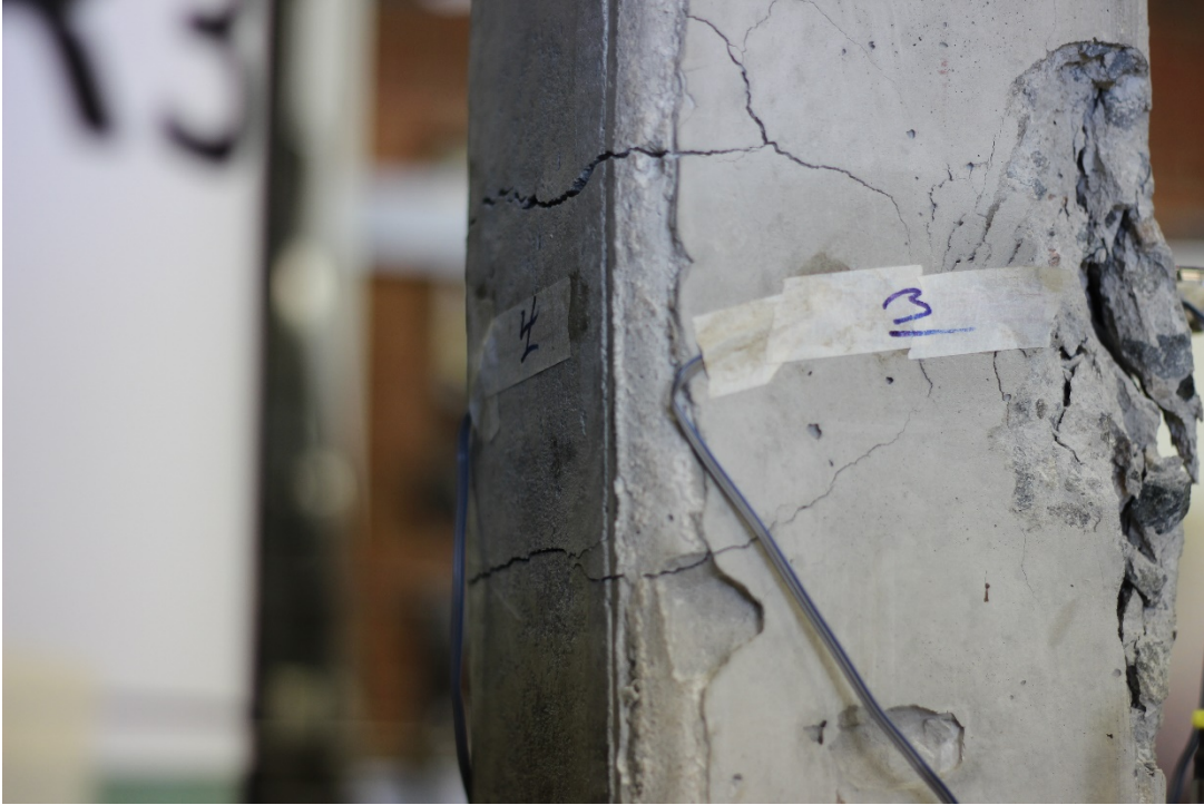
Figure 4.5.1-3 Horizontal tensile cracks in the tension zone of CR3
