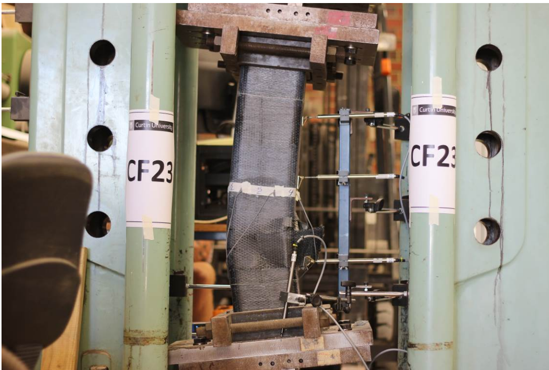
Figure 4.5.1-7 Overall view of CF23 failure
