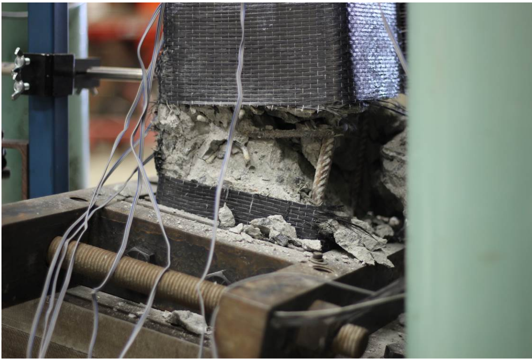
Figure 4.5.1-5 Concrete spalling and rebar rupture in the tension zone of CF13
