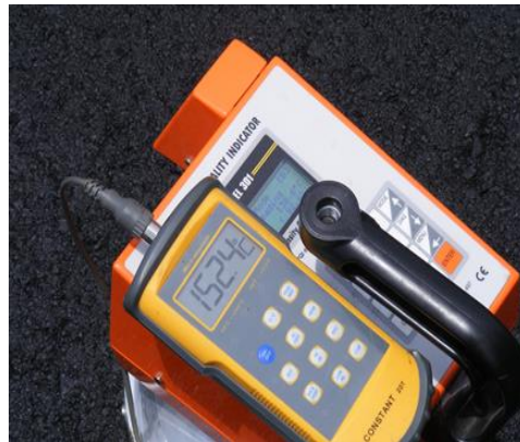
Figure 6.24 HMA surface temperature
