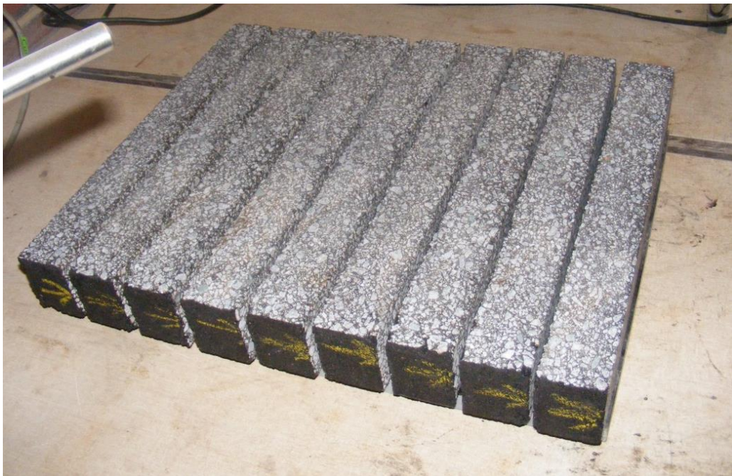
Figure 6.41 Nine beams for fatigue testing
