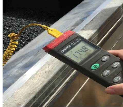
Figure 6.22 HMA temperature in the truck
