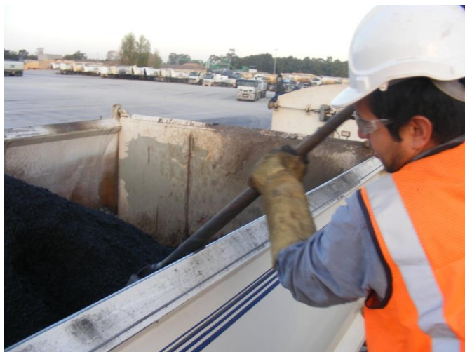
Figure 4.11 Truck asphalt sampling
