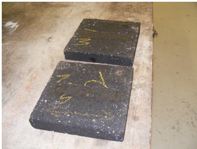
Figure 5.34 Slabs after 10,000 cycles
