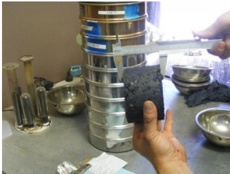
Figure 2.13 Measurement of specimen for bulk density
