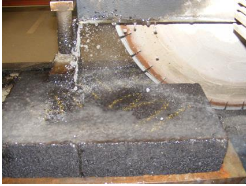
Figure 5.36 Slabs cutting to produce beams
