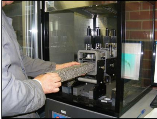
Figure 2.19 Flexural fatigue loading with a warm mix beam
