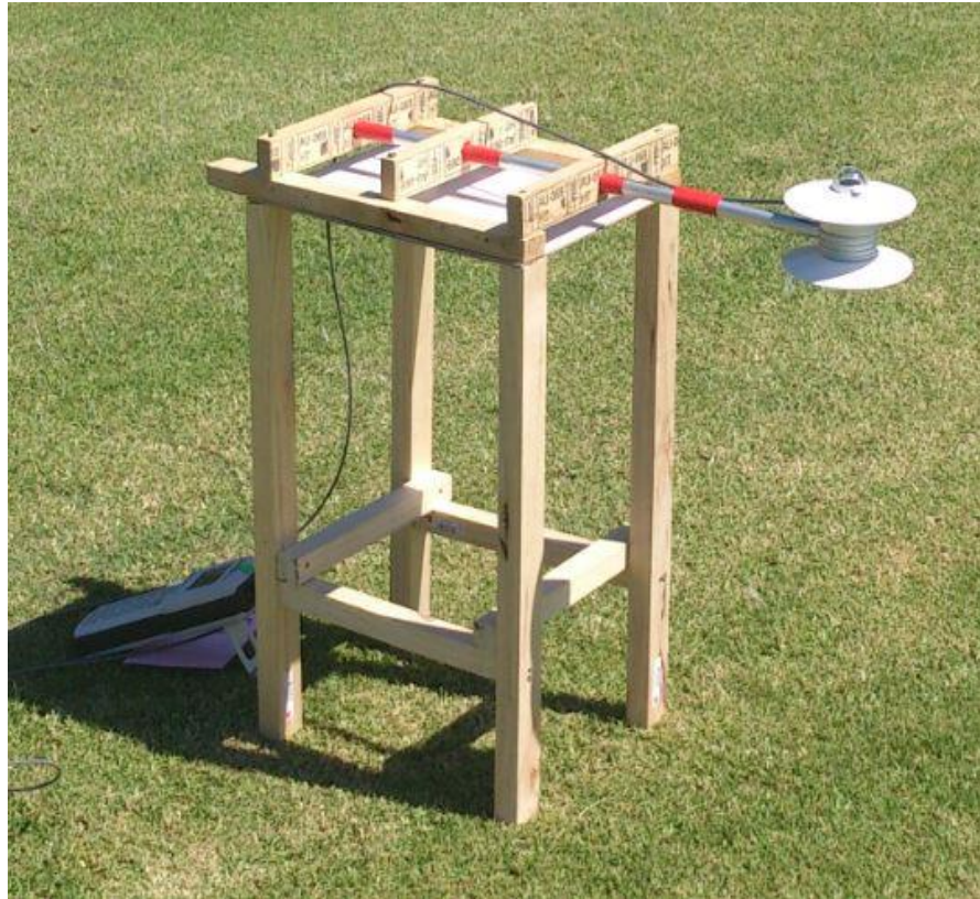
Figure 6.1 Measuring surface albedo by pyranometer with stand at 0.5 m from surface.
