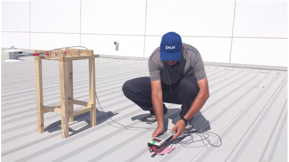
Image showing the Pyranometer instrument used by the author for collecting albedo data in the field, Perth
