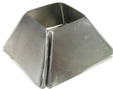
74 Figure 1. Sample of a single unit of truncated square pyramid folded from aluminium sheet 75 (hand folded)
