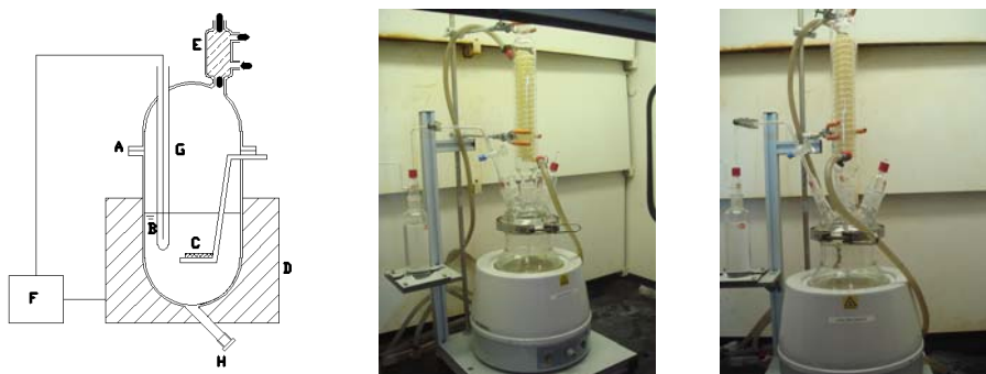
Figure 3-1 Set-up of chemical machining. (A) Glass reaction vessel, (B) solution, (C) substrate holder, (D) Heating mantle, (E) Water-cooled condenser, (F) Temperature controller, (G) Glass encased thermocouple and (H) Outlet Valve.
