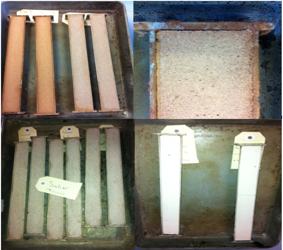
Figure 3.16: Linear shrinkage of pure RCC with different blends of ferricrete and brick and tile after drying in the oven
