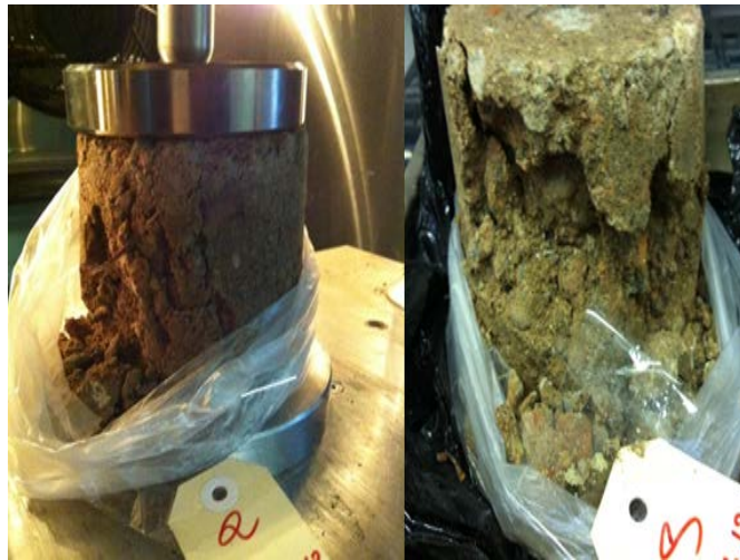
Figure 4.29: Crack patterns in blend of 10% brick and tile with RCC cylinders
