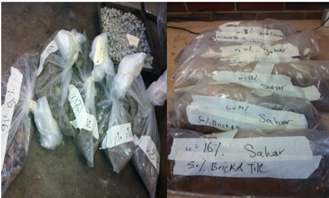
Figure 3.19: Samples prepared and cured for the modified compaction test in this research
