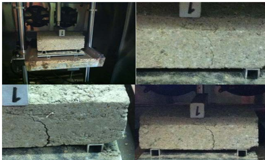
Figure 4.19: Modified bending beam test for beam 4 with support beam
