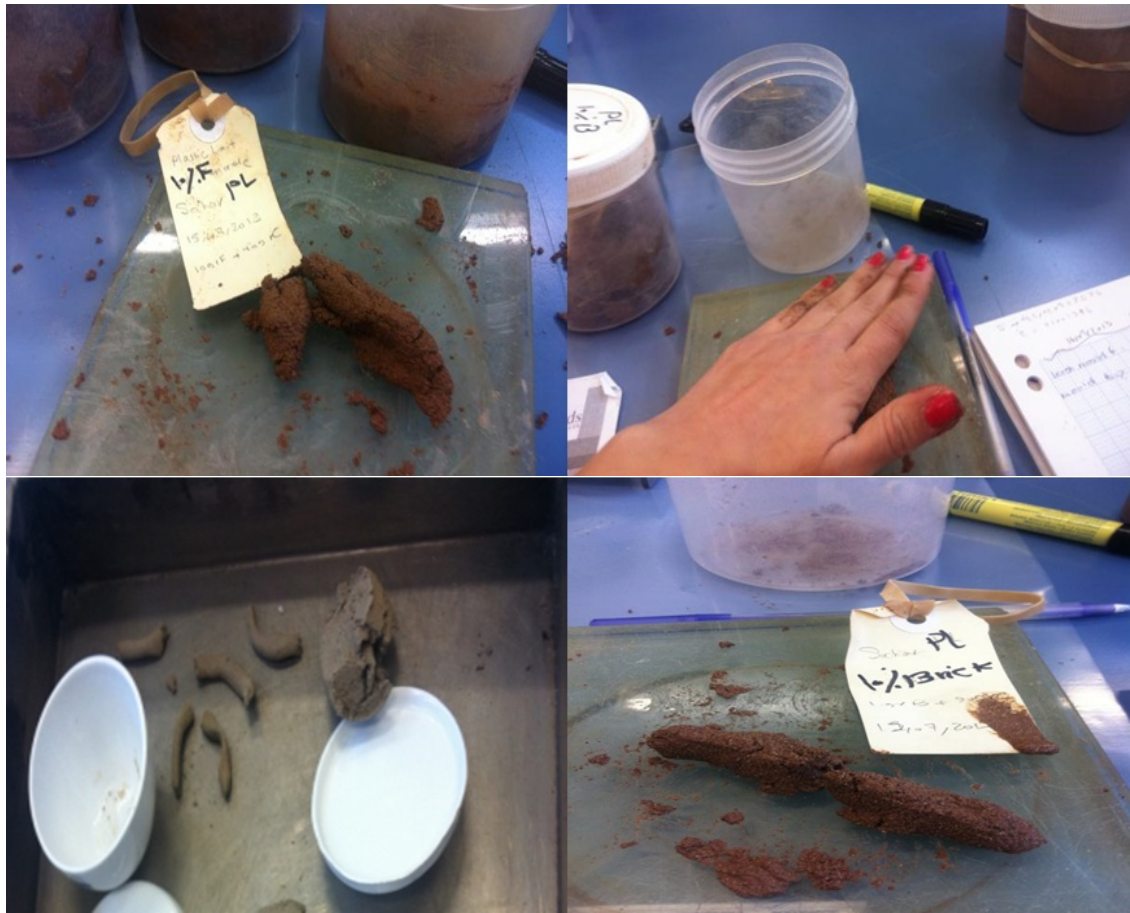
Figure 3.14: Rolling the recycled crushed concrete to form a 3 mm diameter thread with crumbling
