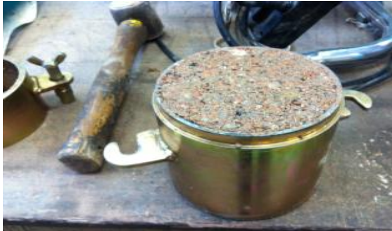
Figure 3.23: Compacted RCC core
