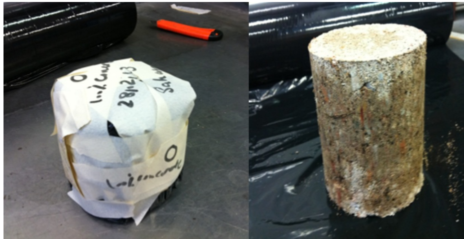
Figure 3. 27: Wrapping the cores
