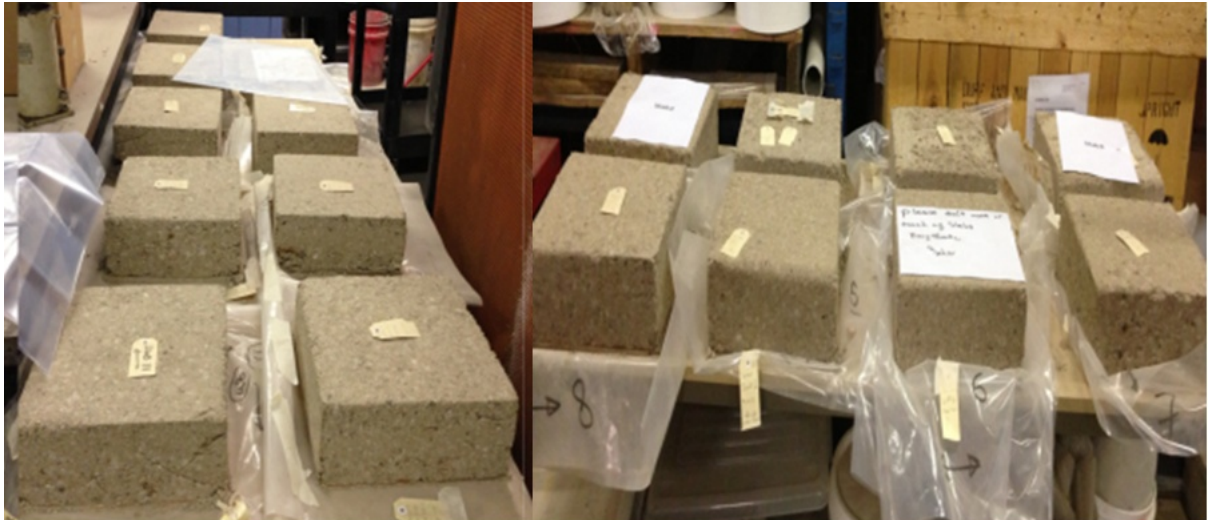
Figure 3.34: Curing and storing the slabs for 56 days
