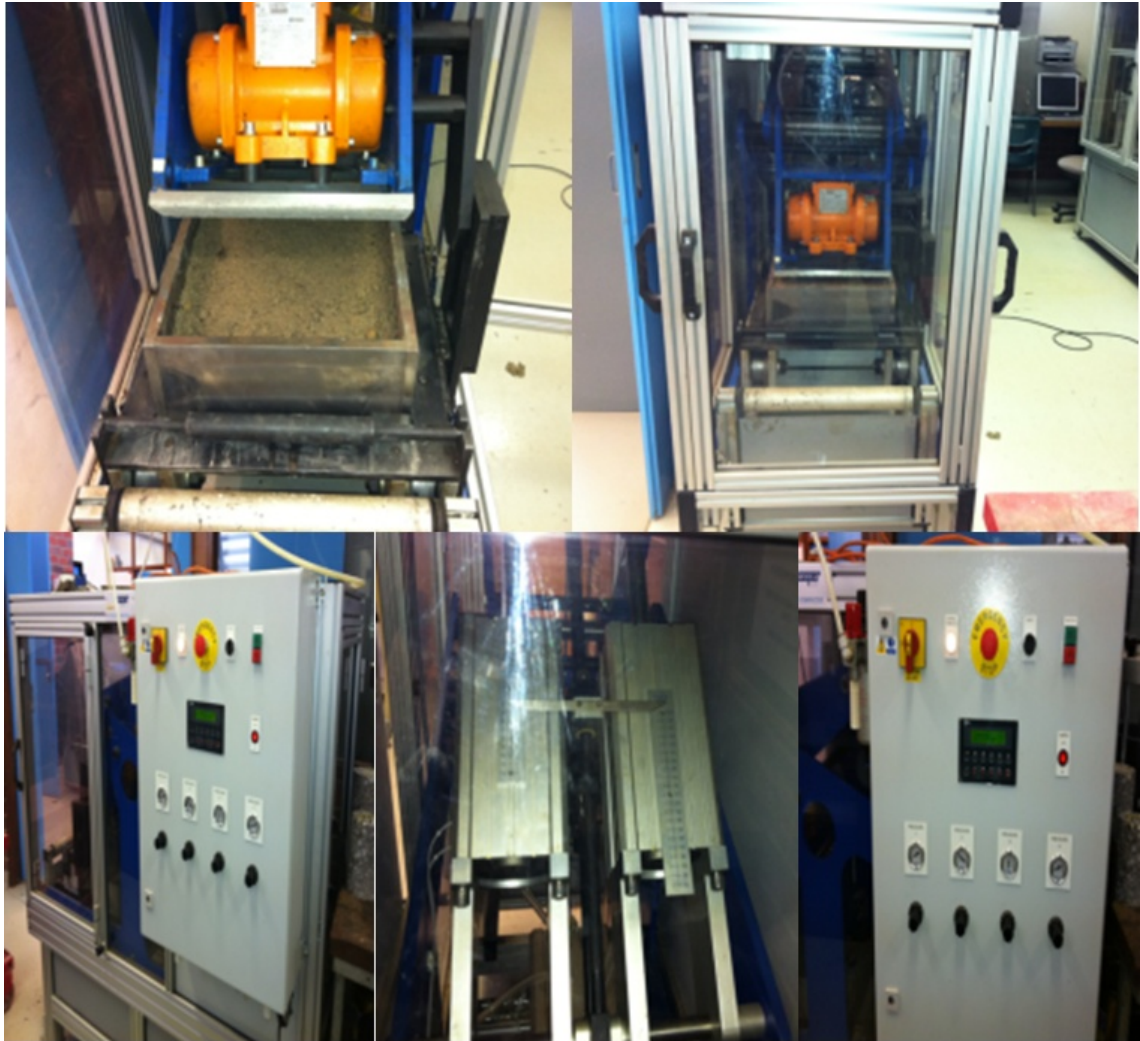
Figure 3.33: Cooper compactor device used for compacting the slabs
