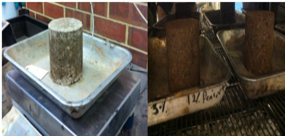
Figure 3. 26:: Cores dried back to 60% OMC
