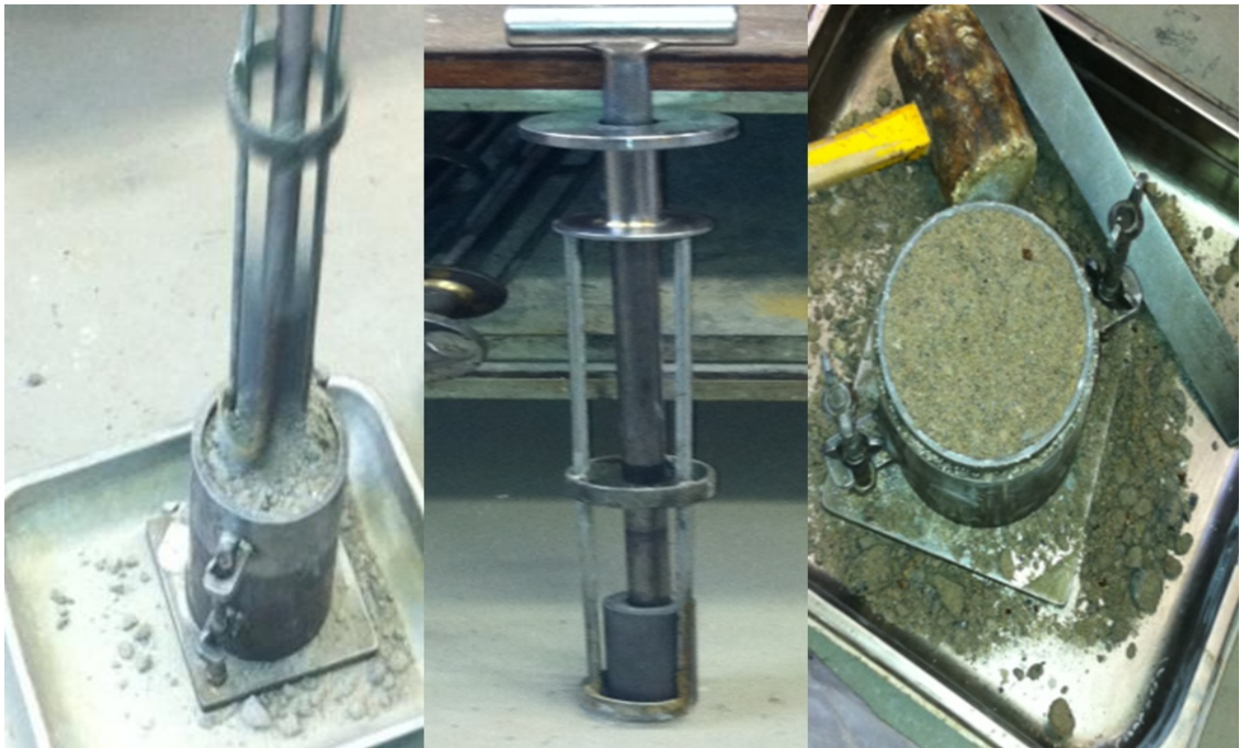
Figure 3.17: Modified compaction equipment
