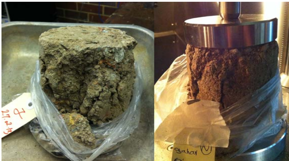
Figure 4.28: Crack patterns in pure RCC cylinders
