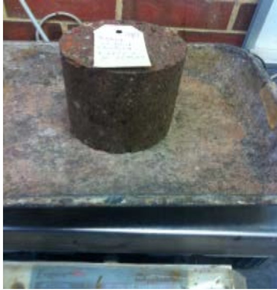
Figure 3.25 : Wet compacted cores
