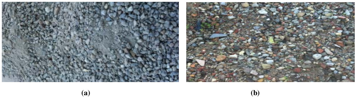
Figure 3.5: (a) Recycled crushed concrete (RCC) (b) Commingled brick and tile with RCC used in this research
