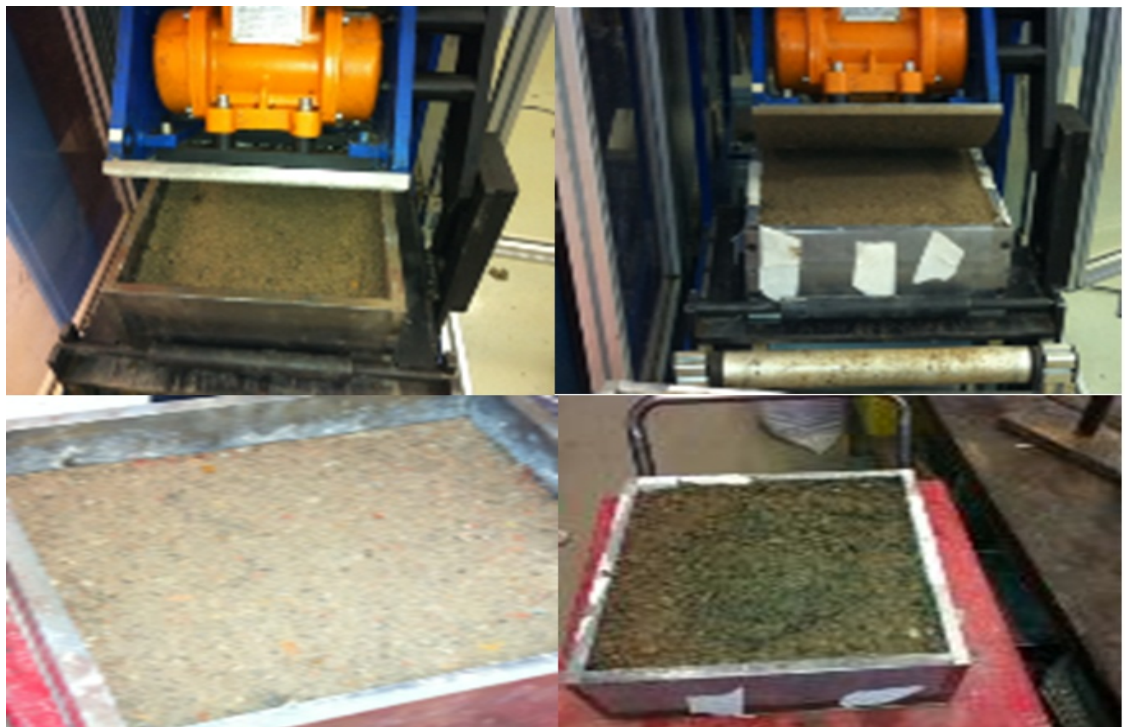
(a): Compaction of RCC slabs to a height of 7.5 cm (b): Compaction of RCC slabs to a height of 115 cm
