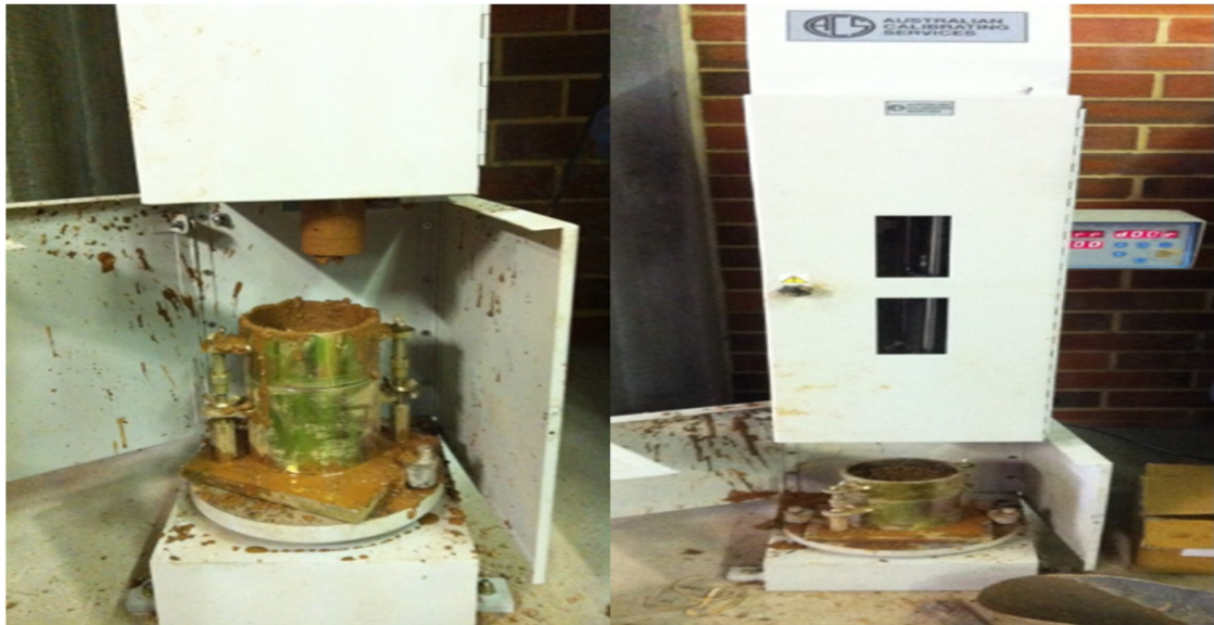
Figure 3.18: Modified Compaction process by the automatic soil compactor machine
