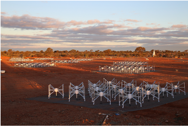
Figure 1. MWA Phase II tiles in the Murchison Radio-Astronomy Observatory in Western Australia. (Taken by Greg Rowbotham in June 2016 when Phase II was under construction.)
