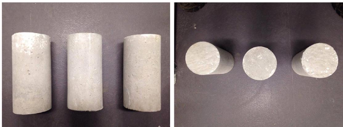
Figure 7. Physical appearance of PC-FNS100 samples after wet-dry cycles
