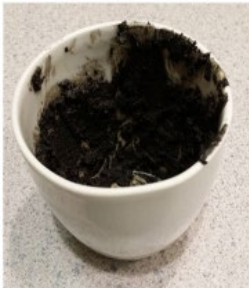
Unroasted sticky paste-like material derived from ground run-of-mine ore mixed with \text{H}_2\text{SO}_4 , \text{CaCl}_2 or \text{MgCl}_2
