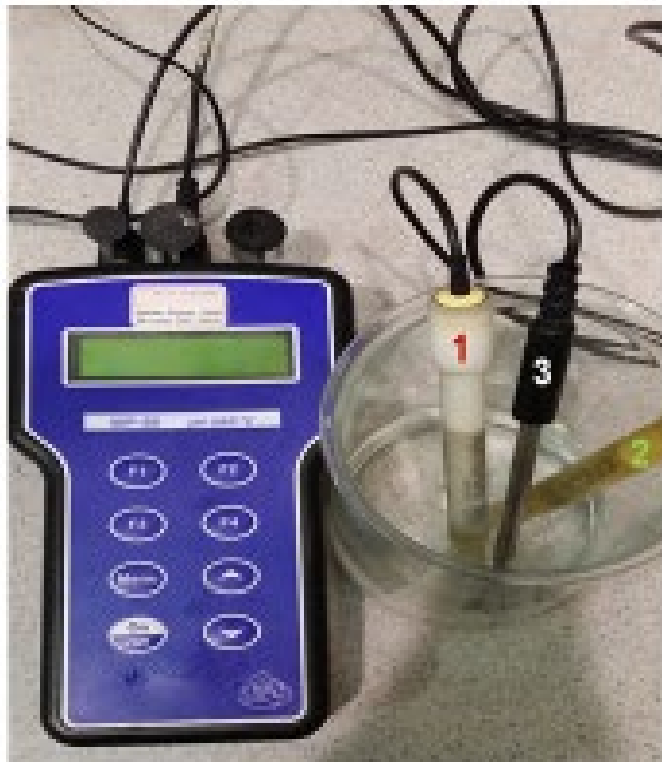
pH meter WP-80 with probes (1), (2) and (3) for measuring solution pH, Eh and temperature
