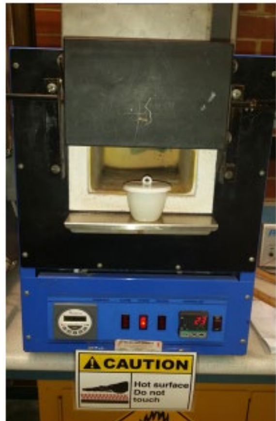
Static-air muffle furnace equipped with a programmable temperature controller
