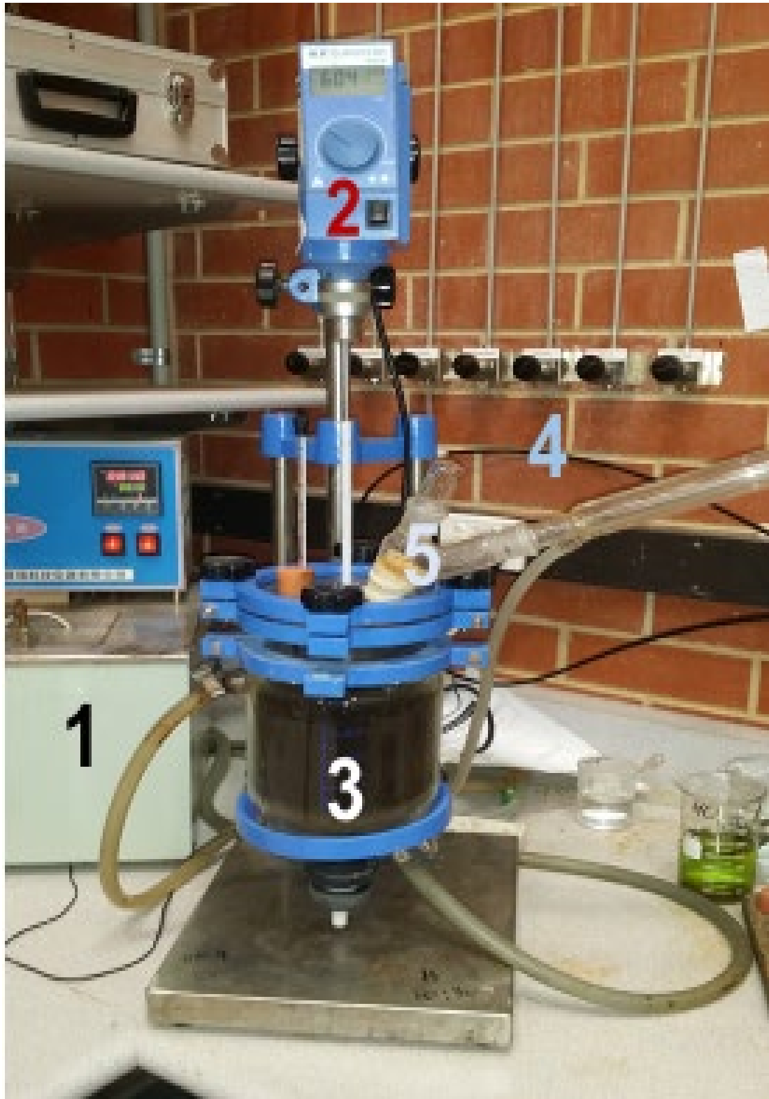
Experimental setup at leaching stage: (1) Thermostated water-bath, (2) IKA Eurostar variable speed overhead mechanical stirrer (3) Batch reactor with conical bottom (4) Transfer tube for adding oxygen, (5) Cooling reflux condenser connected to a chilled water line
