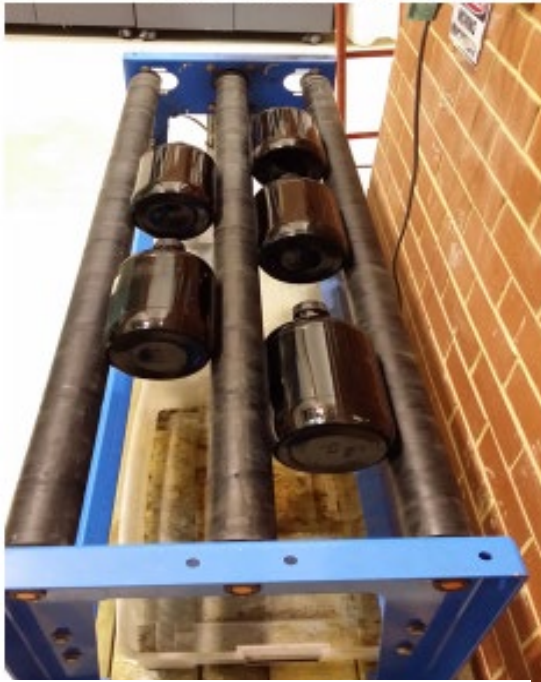
Experimental setup at adsorption stage: Open-ended rolling bottles rotated at 105 rpm
