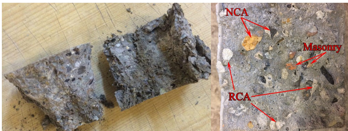
Figure 4. Geopolymer sample containing RCA after testing.
