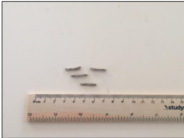
Fig. 2.4. Bulk continuous filament (BCF) as a typical geo-synthesis used in soil reinforcement ( Chegenizadeh et al. 2018a )
