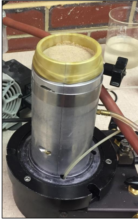
Fig. 6.8. A typical specimen during preparation in split mould.
