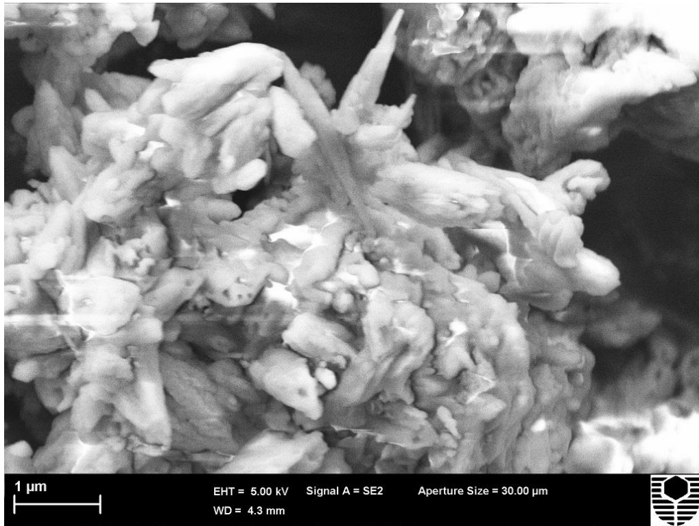
Fig. 2.7. A typical scanning electron microscopy (SEM) of the lime
