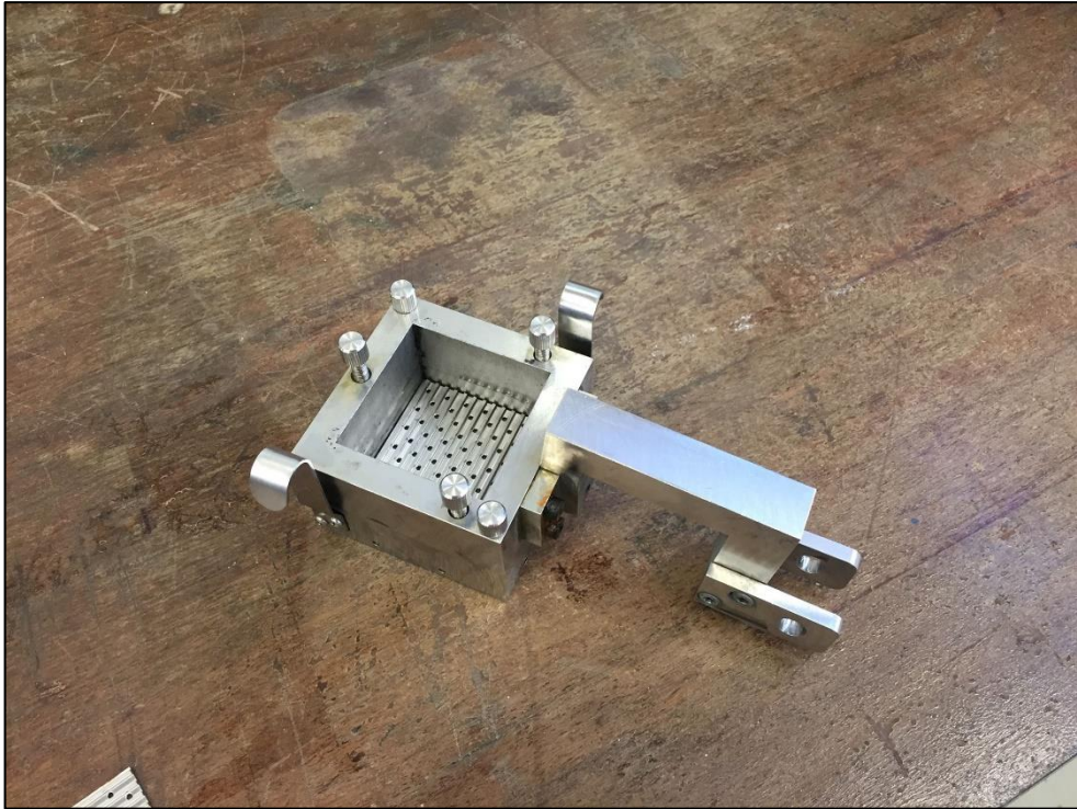
Fig. 3.1. The sample container in direct shear test
