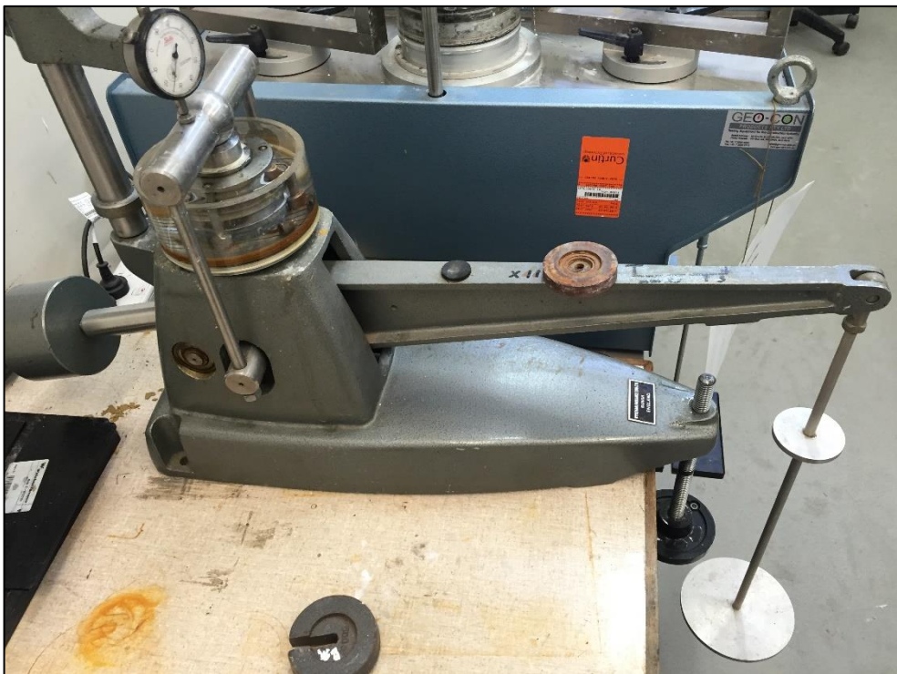
Fig. 3.6. An oedometer device to measure the consolidation of the sample
