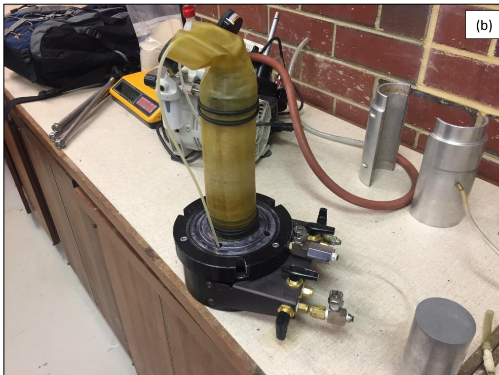
Fig. 3.10. Sample preparation in a triaxial device using moist tamping method (a) Sample preparation in a steel split mould; and (b) prepared sample on pedestal and ready for the tests.
