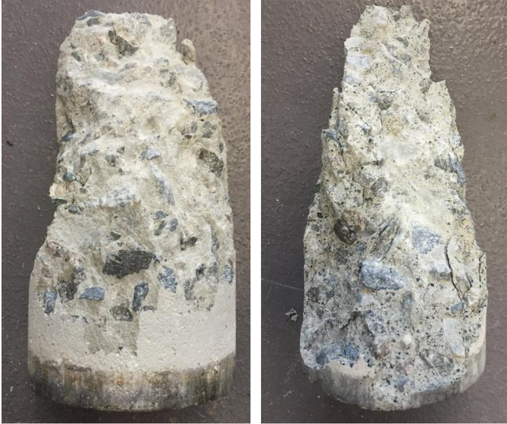
Fig. A.12 Similar failure pattern of control concrete (left) and FNS concrete (right)
