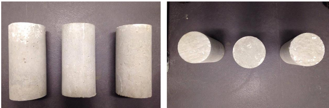
Fig. 7.4 Physical appearance of PC-FNS100 samples after wet dry cycles
