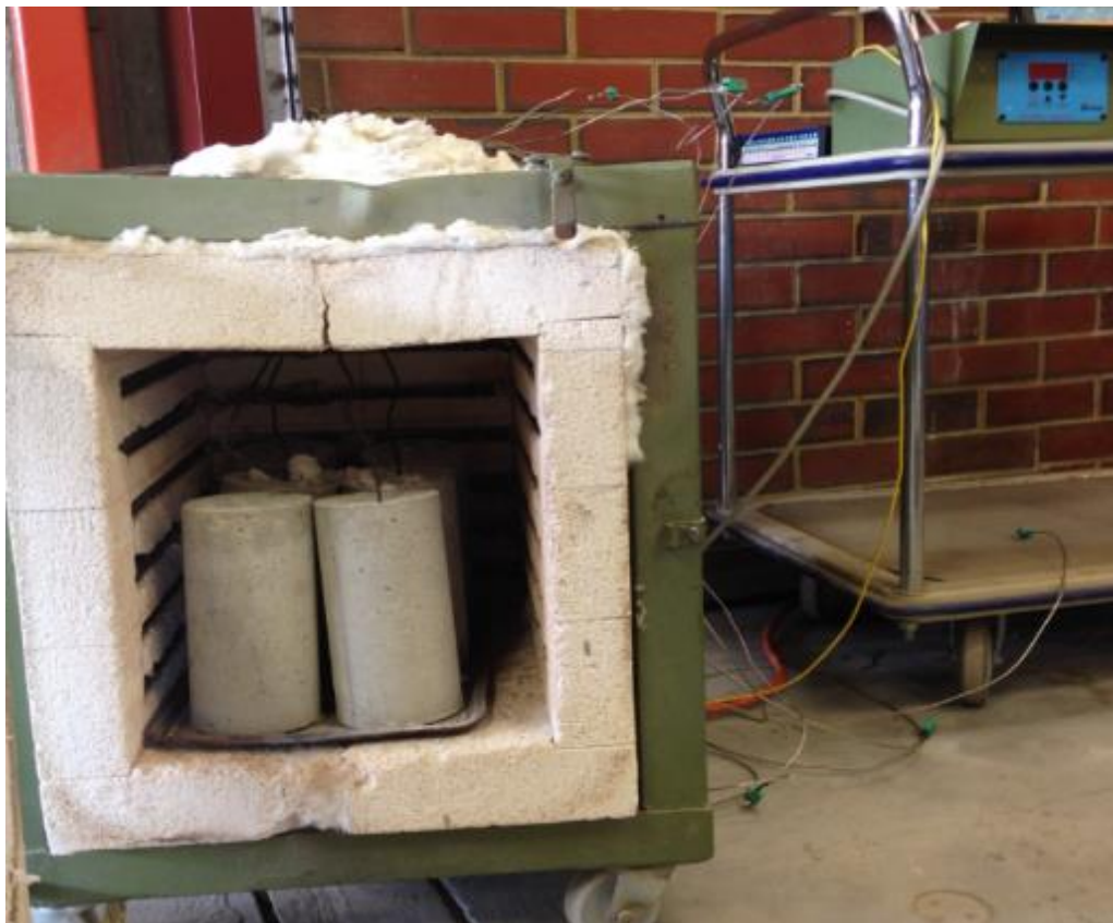
Fig. A.10 Elevated temperature exposure test
