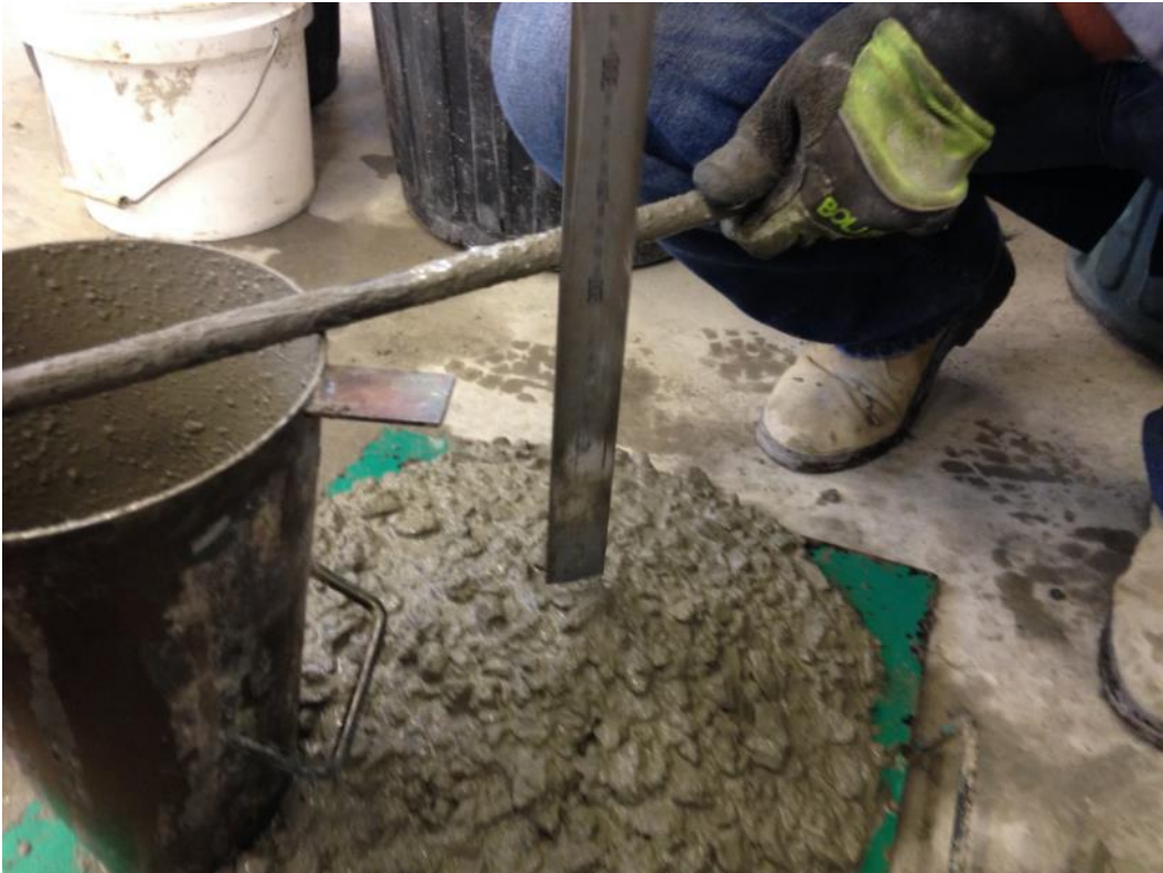
Fig. A.1 Slump test of concrete
