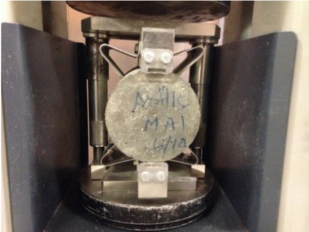
Fig. A.5 Splitting tensile strength test of concrete
