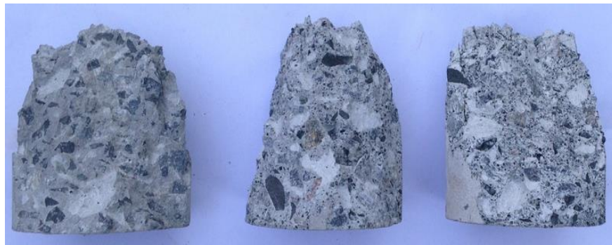
Fig. 4.5 Samples after compressive strength test (left: PC-FNS0, middle: PC-FNS50 right: PC-FNS100)
