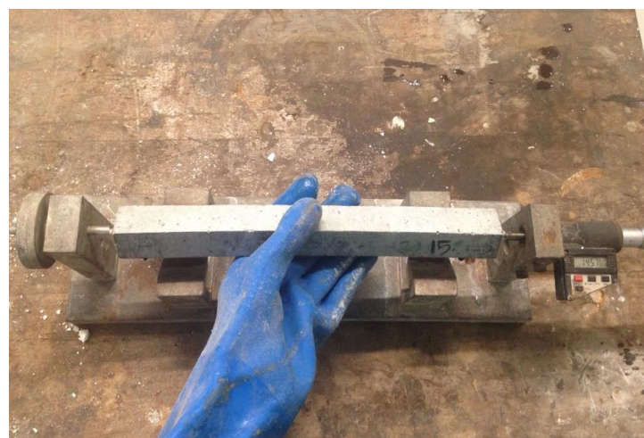
Fig. 6.1 Length measurement of a mortar bar specimen
