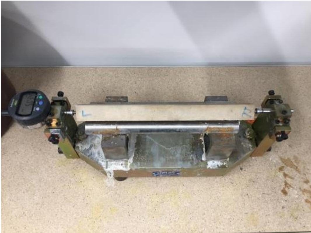
Fig. A.9 ASR expansion measurement by length comparator
