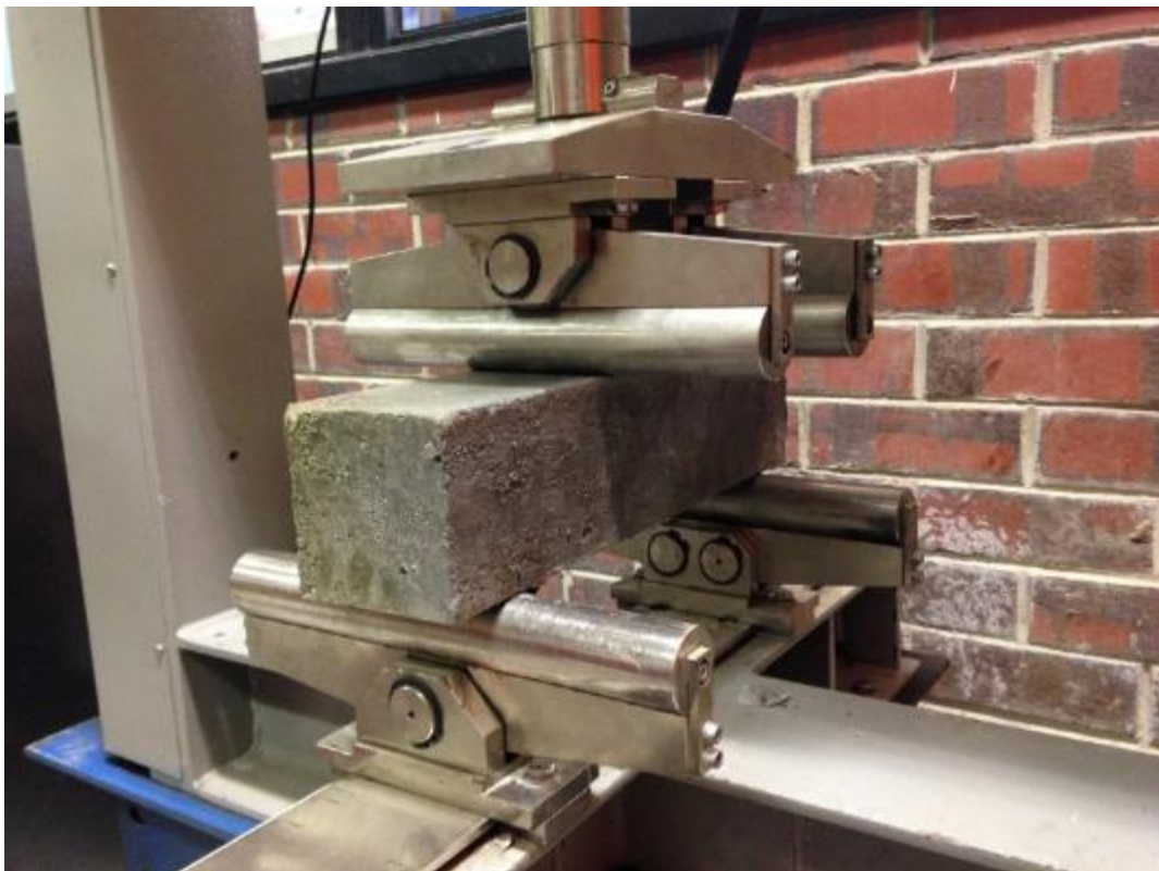
Fig. A.6 Flexure strength test of concrete
