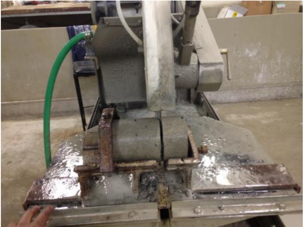
Fig. A.7 Concrete cylinders cutting for RCPT and sorptivity tests
