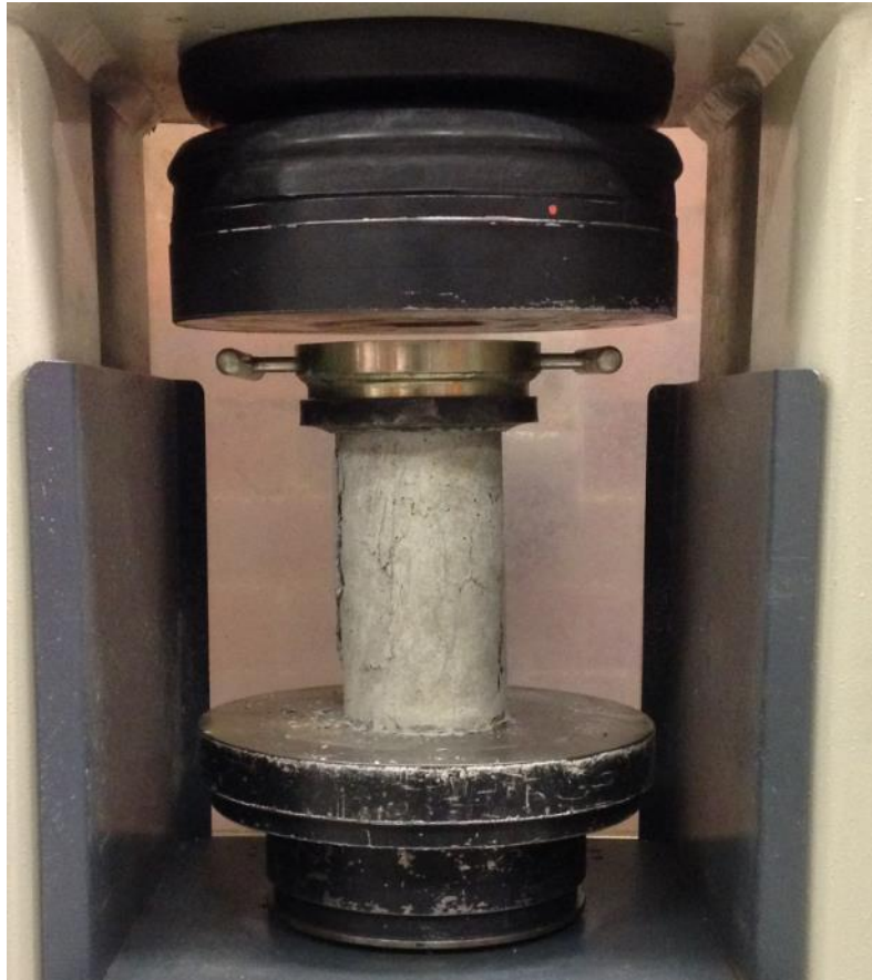
Fig. A.3 Compressive strength test of concrete
