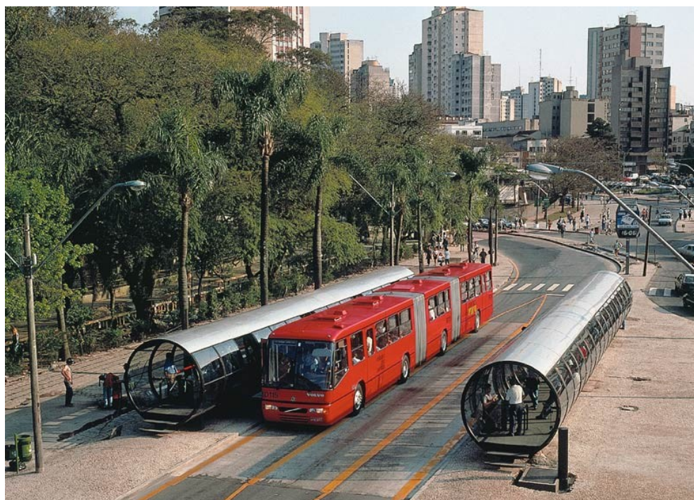
Plate 2.2: A Bi-articulated Bus on the Curitiba BRT System 60
