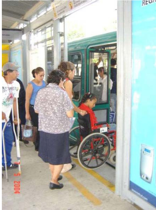
Plate 2.4: Level Boarding on the Optibus BRT system 67
