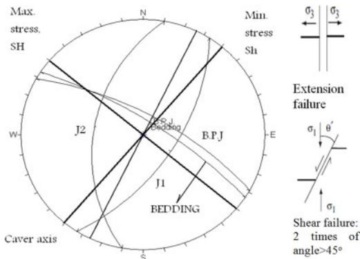
Figure 3. The direction of max. and min. horizontal stresses, cavern direction, all joint sets and direction of stress proportionate shear and dilational fractures.
