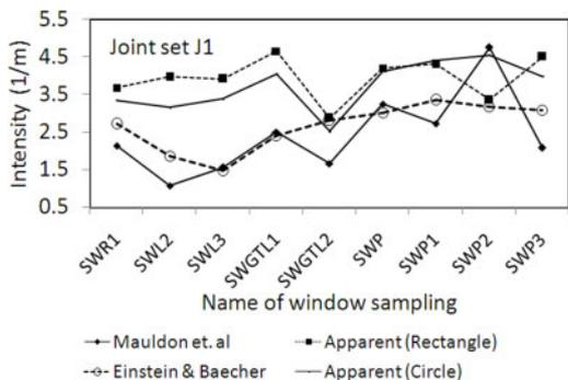
Figure 4. The actual and apparent areal intensity of J1 joint set.
