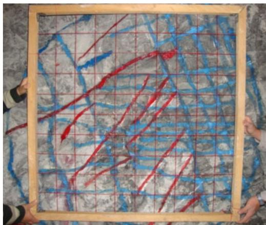
Figure 5. The window sampling with 10\*10 cm grids in SWL2 location.
