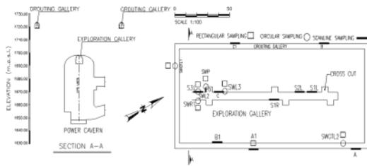
Figure 1. Location of exploratory gallery in cavern roof and cavern peripheral gallery with the location of scanlines and areal sampling.
