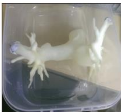
Figure 2: Three-dimensional printed pulmonary model is placed in a plastic box which is used to be filled with contrast medium for computed tomography scans
