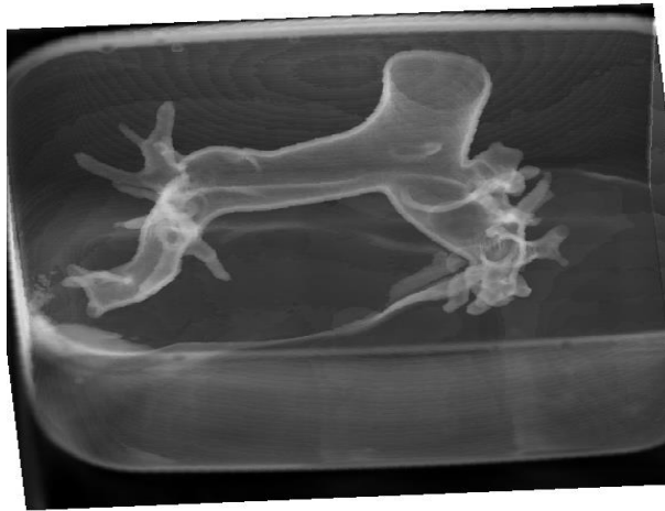
Figure 5.2 3D visualization of 3D printed pulmonary artery model which was placed inside the container filled with contrast medium. Since the model was immersed into the water with diluted contrast medium with similar CT attenuation to that of routine CT pulmonary angiography, surface voxel projection was used to create 3D view of the model.
