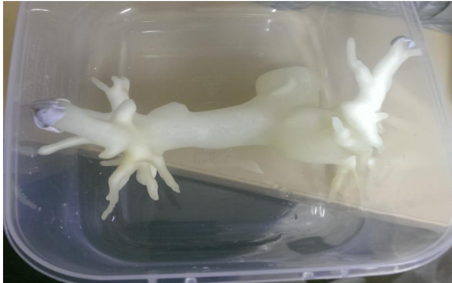
Figure 3.2 3D printed pulmonary model is placed in a plastic box which is used to be filled with contrast medium for CT scans.
