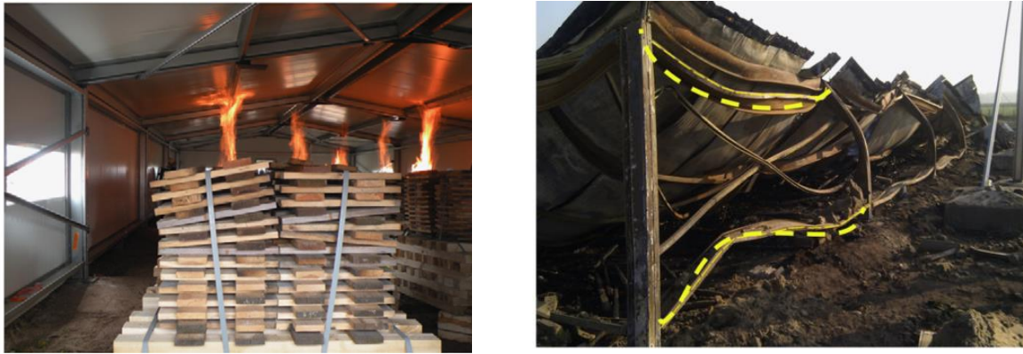
Figure 2.11: During Fire Test and After Fire Test (Pyl et al. , 2012)
