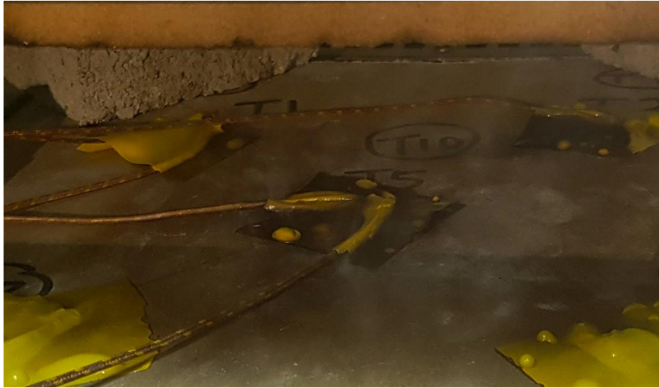
Figure E.10 Initiation of Charring of Gypsum Board (Specimen 2)
