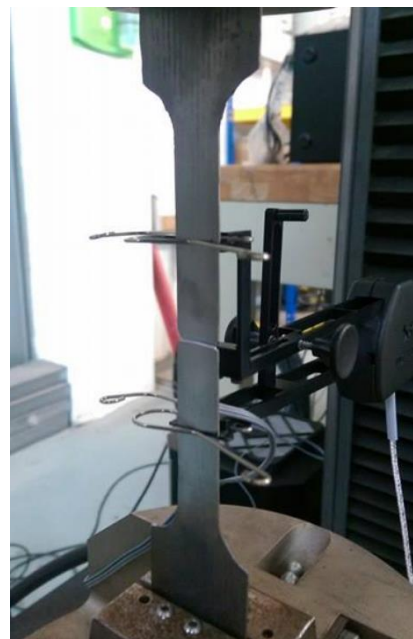
Figure 4.3: Failure of a Coupon Specimen
