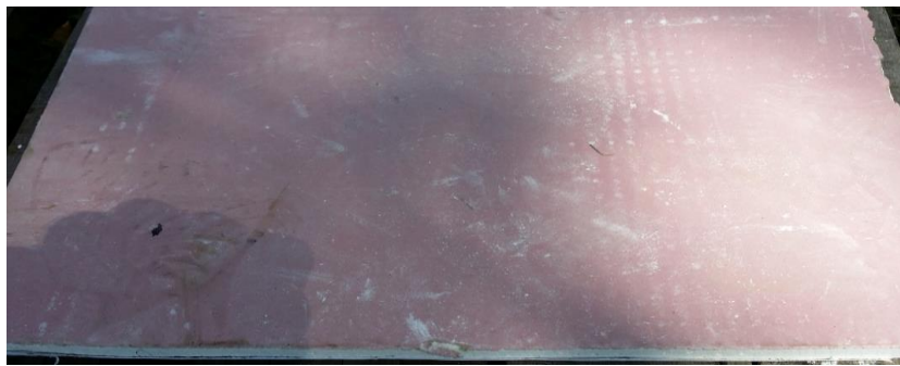
Figure 3.35: 15 mm Gyproc Fireline Gypsum Board
