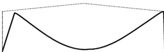
Figure 2.6: Inward Collapse (O’Meagher et al. , 1992)
