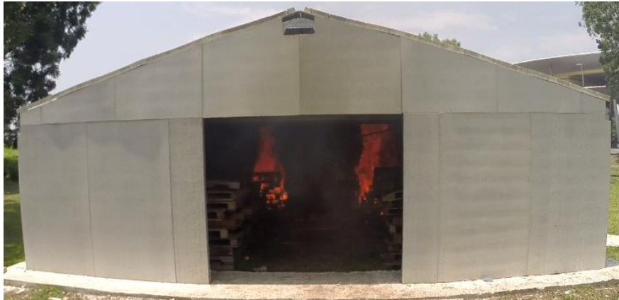
Figure 6.5: Fire Test at 13 minutes 37 Seconds
