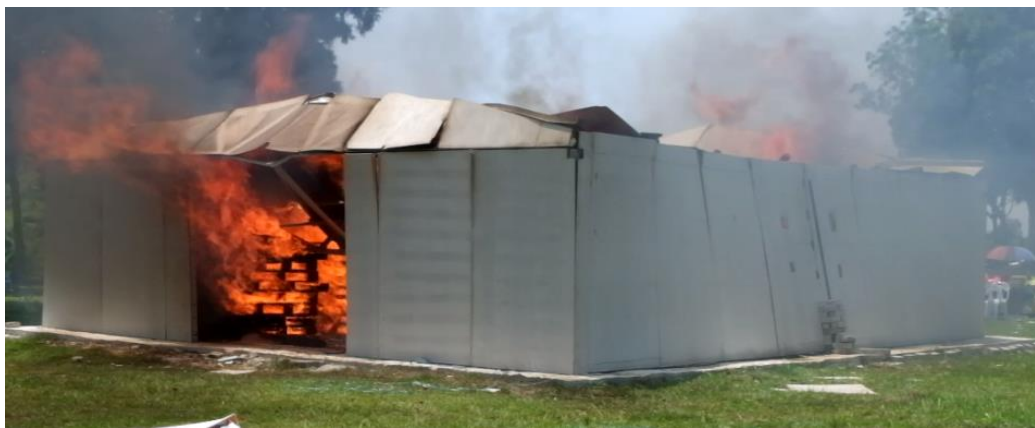
Figure 6.10: Fire Test at 22 Minutes
