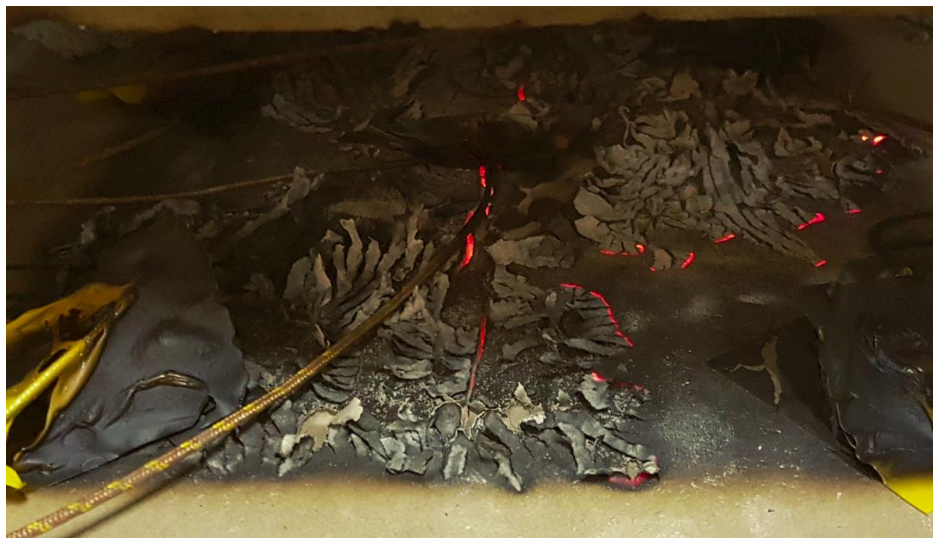
Figure E.11 Cracks Developed on Ambient Surface of Gypsum Board (Specimen 2)
