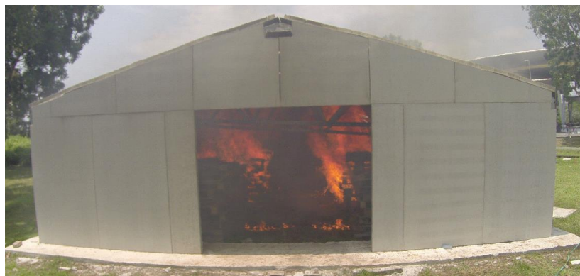
Figure 6.24: Mode of Collapse in Full-Scale Fire Test (Apex Temperature at 583 °C)
