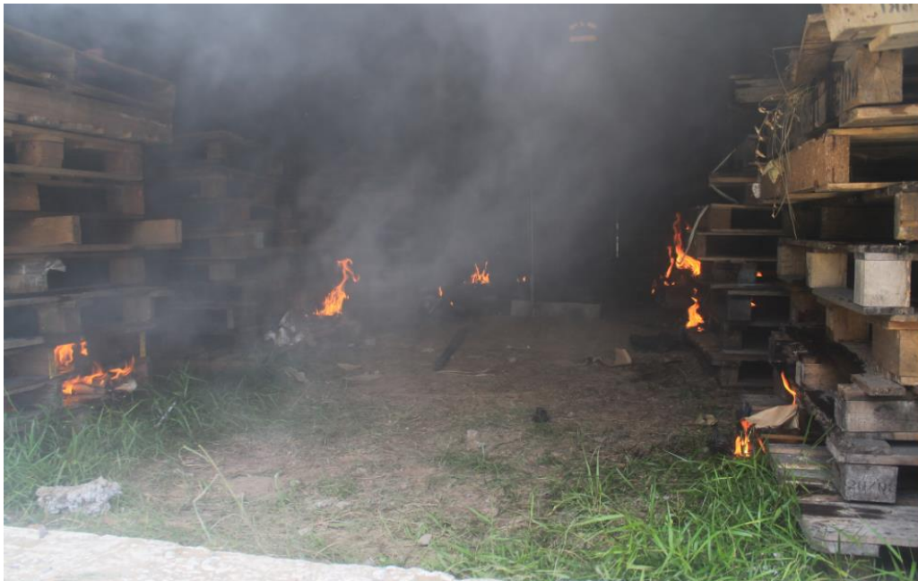
Figure 6.2: Ignition Stage (120 second)
