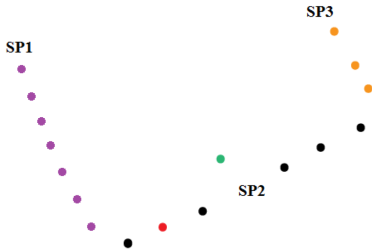
Figure 3.3 Example of direction vector estimation, different colours indicate different scan profiles: purple points are points of scan profile SP1; Black points and the red point are points of scan profile SP2; Orange points are points of scan profile SP3 and green point is outlier points; the red point is the query point.
