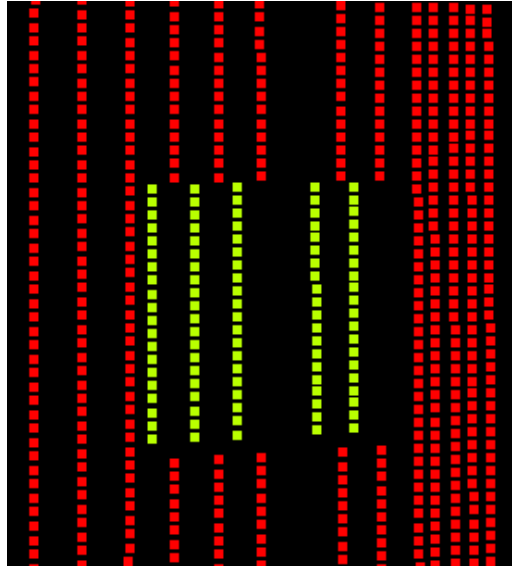
Figure 2.9 Examples of scan profiles of a building façade (red) and a window (yellow)
