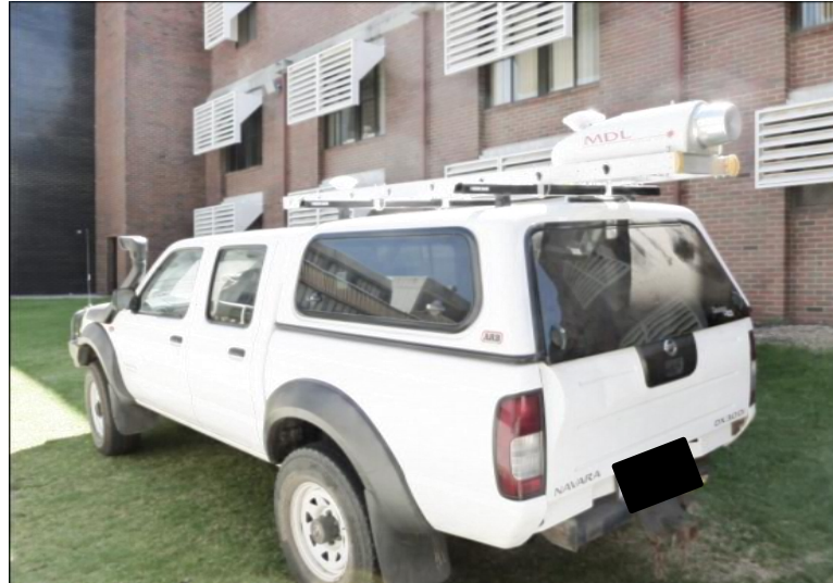
Figure 1.1 An example of a MLS system – MDL Dynascan S250 mounted on a car
