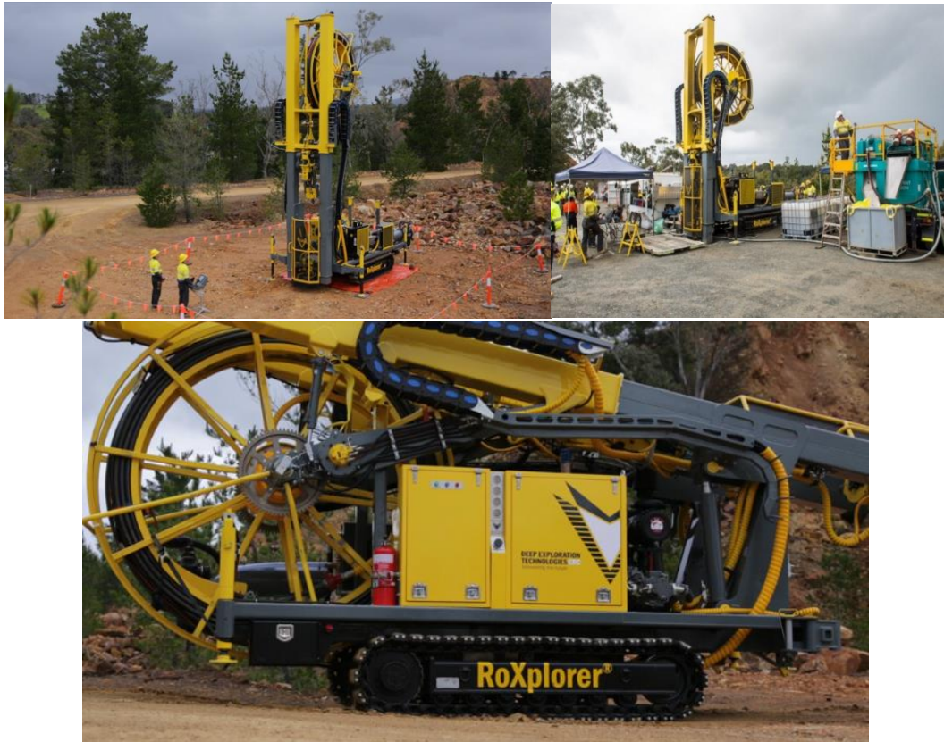
Figure 55. Coiled tube drilling system, RoXplorer, used in the drilling trials in South Australia - courtesy DET CRC.
