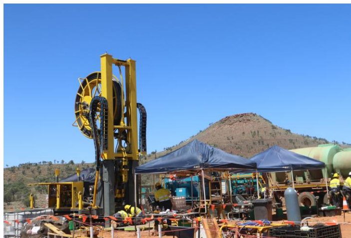
Figure 48. Field trial of RoXplorer Coiled Tubing rig at Port Augusta - Photo courtesy of DET CRC.
