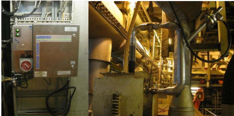
Figure 31. (Left) FRM electronics box and purge unit; (Right) FBRM apparatus and pipe-mounting adapter [75].
