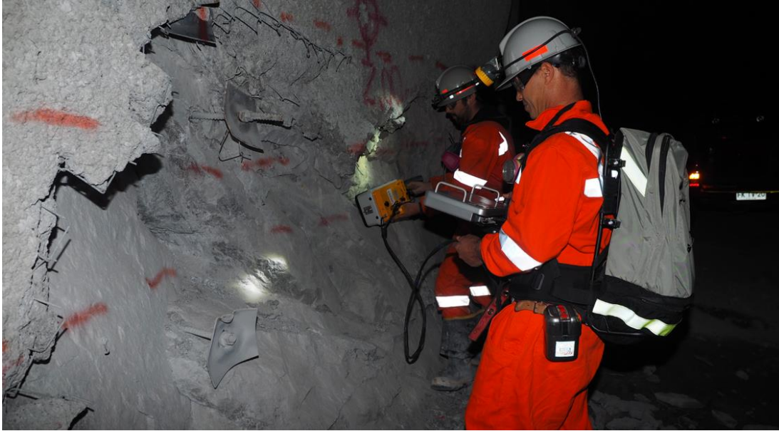
Figure 355 - GPR survey of the rock mass following simulated destressing blast damage.
