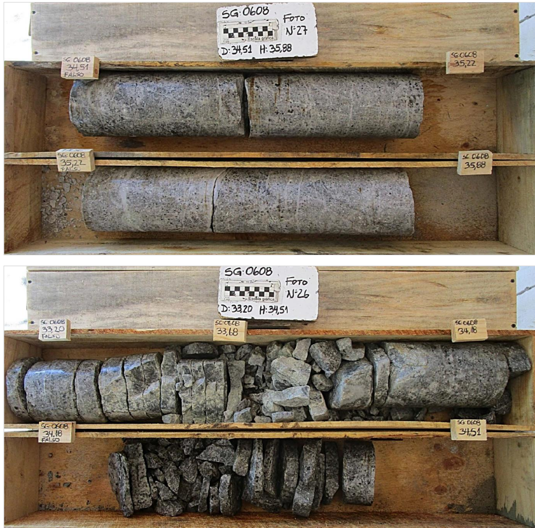
Figure 72 - Examples of intact and stress-damaged disking core taken from the pilot boreholes.
