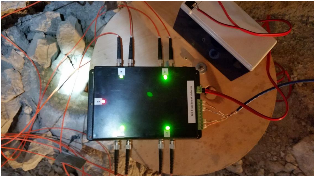
Figure 238 - Fibre optic break reader used to correlate detonator initiation to seismic system timing.
