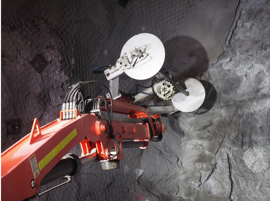
Figure 198 - Mesh handler arm for mechanised ground support installation (mesh roll not shown).
