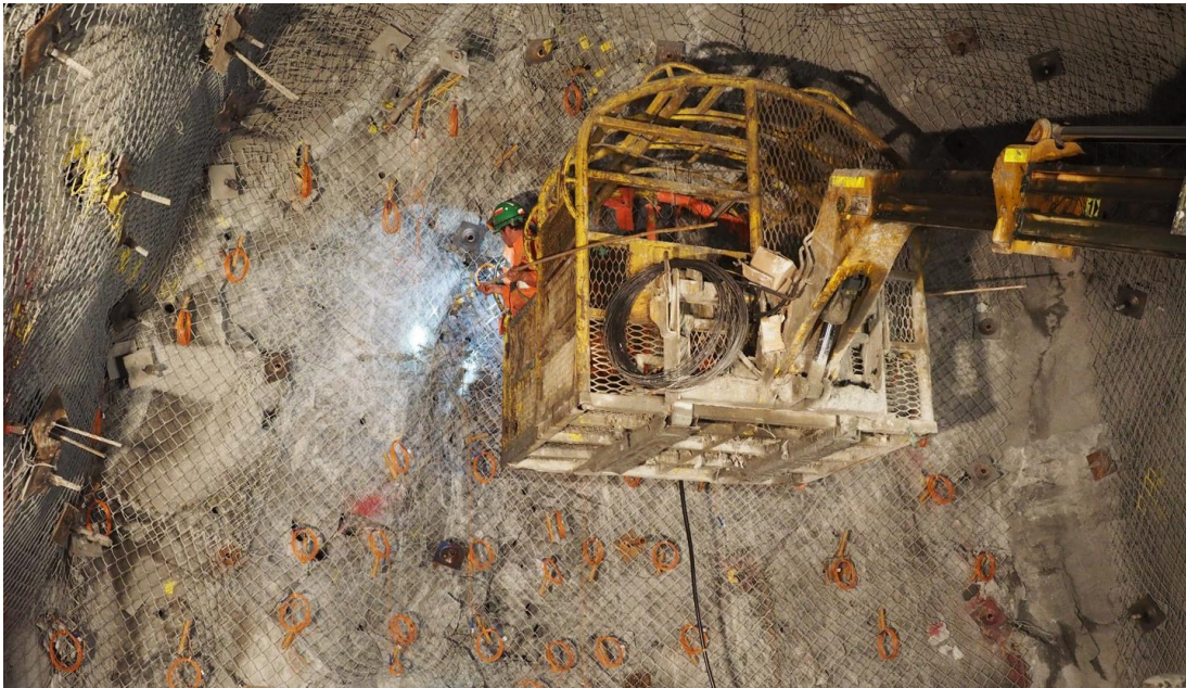
Figure 182 – Insertion of the Tronex collar primer for a destressing charge.
