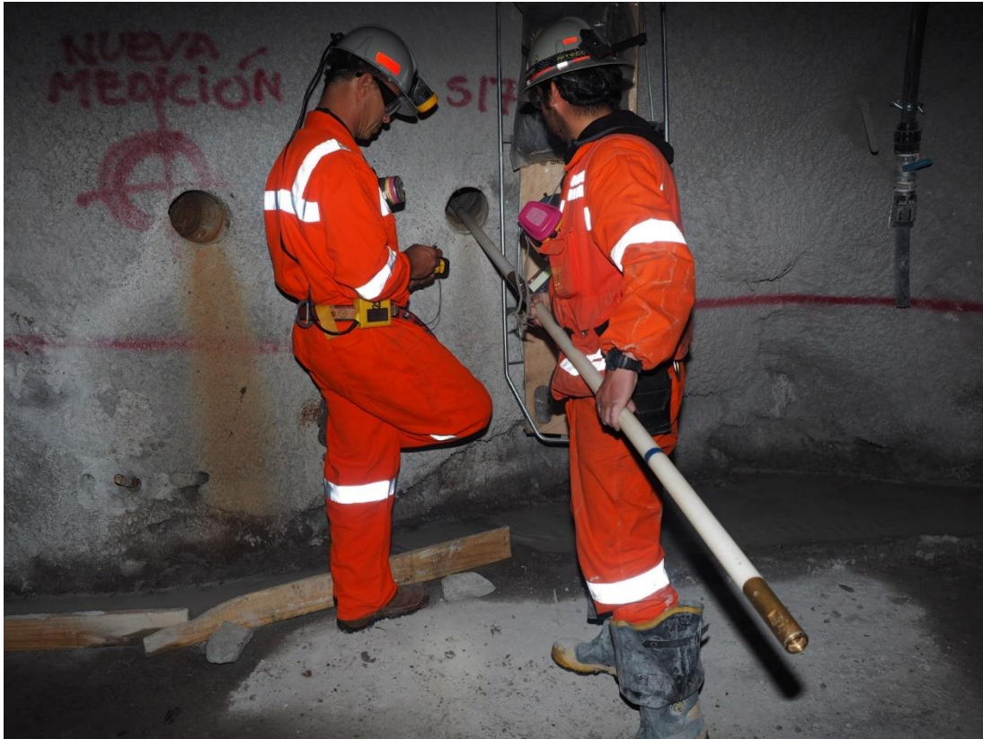
Figure 352 - Borehole radar survey.
