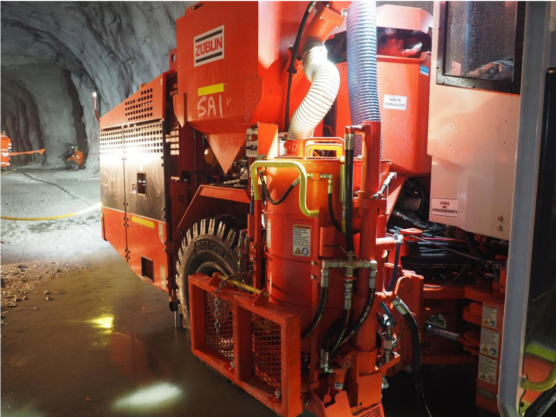
Figure 197 - Integrated grout mixing bowl on the mechanised ground support jumbo.
