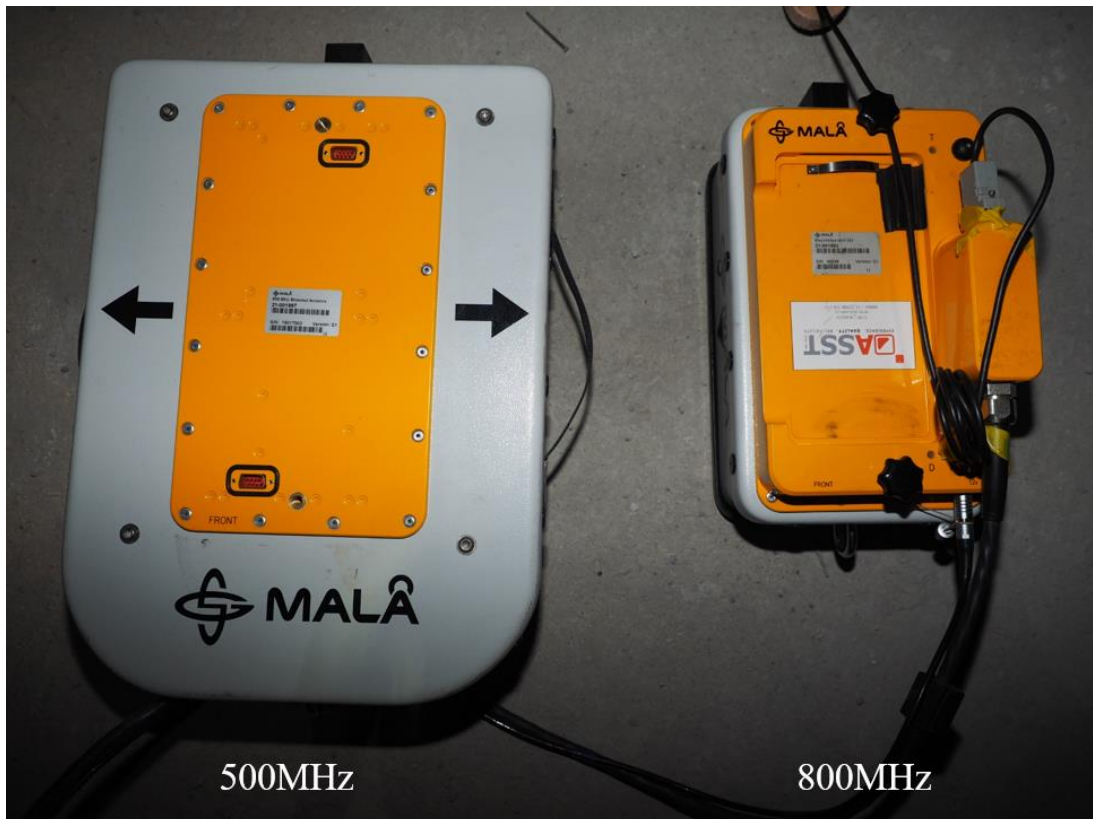
Figure 349 - Surface monostatic ground penetrating radars in 500MHz and 800MHz frequency.
