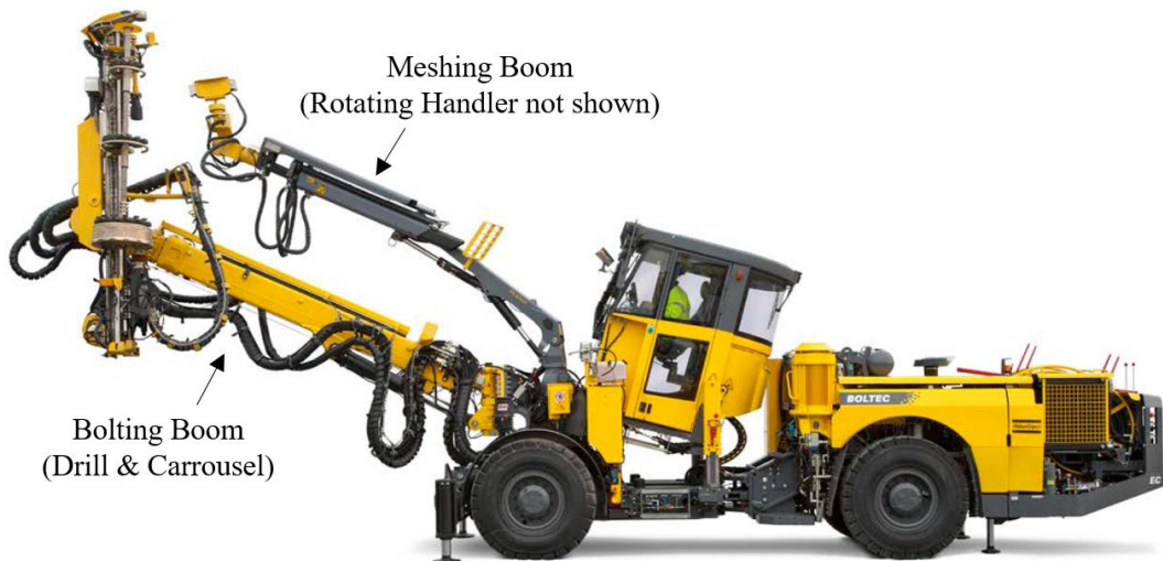
Figure 192 – Mechanised Boltec jumbo used for ground support installations (AtlasCopco, 2017).
