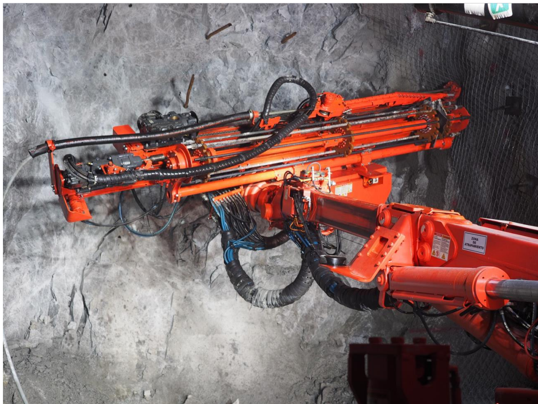
Figure 195 – Mechanised jumbo boom for drilling, grouting and installing reinforcement.
