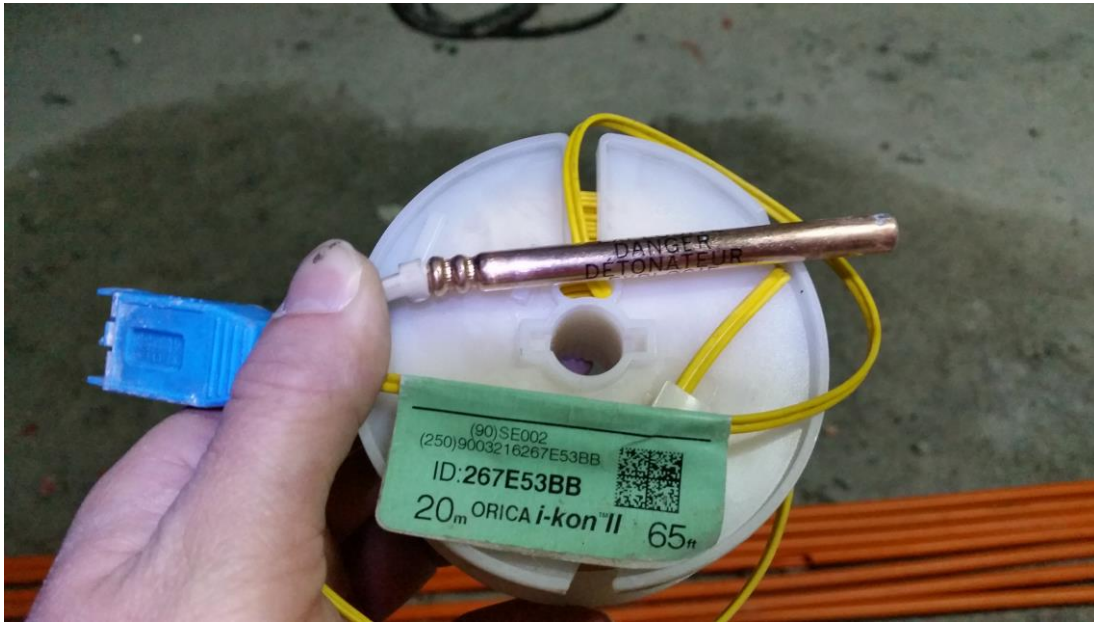
Figure 234 - Electronic iKon detonator used as an artificial seismic source for velocity calibration.
