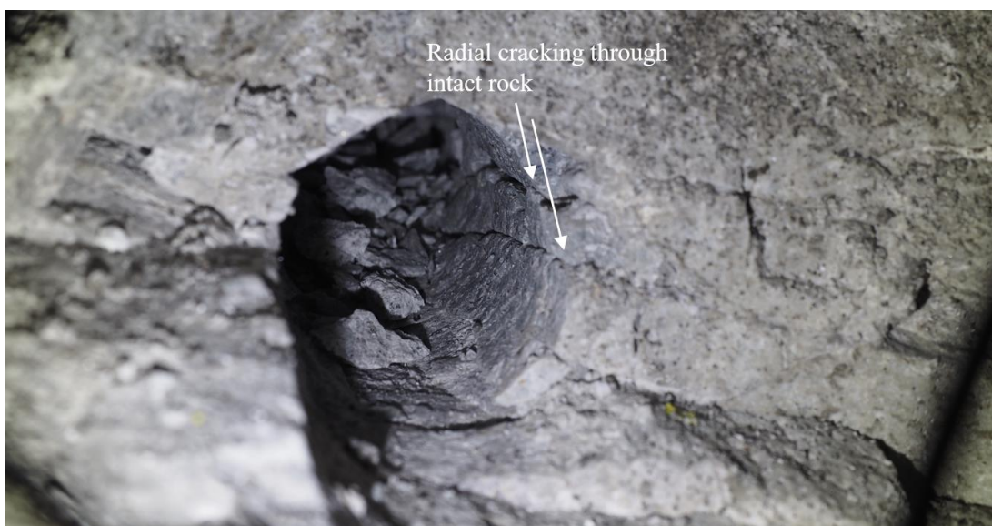
Figure 329 - Borehole internal view of radial fracturing through intact rock (opposite direction).
