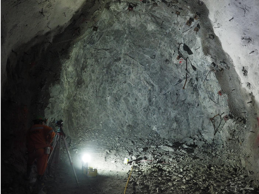
Figure 189 - Typical digital photogrammetry station for face structural mapping.
