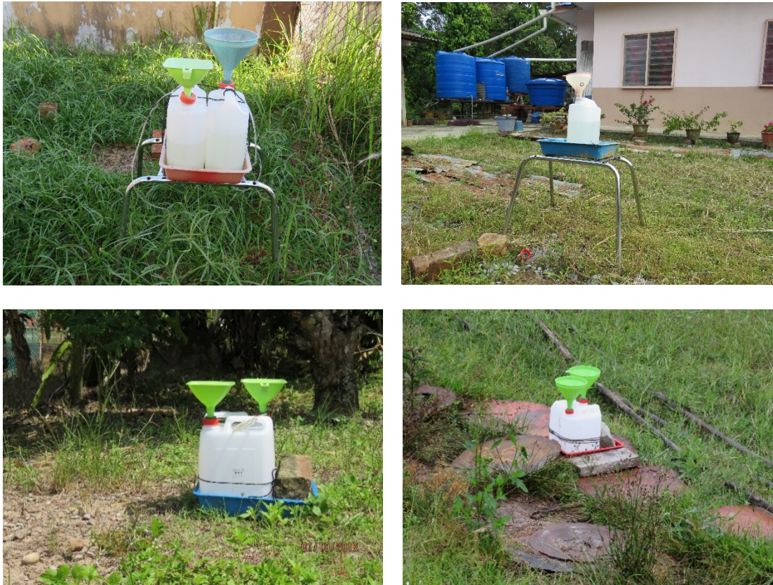
Figure 3.3: Experimental set up for cumulative sampling of precipitation for isotopic analysis (retrieved from IAEA, (1997), Technical Procedure for cumulative monthly sampling of precipitation for isotopic analysis).
