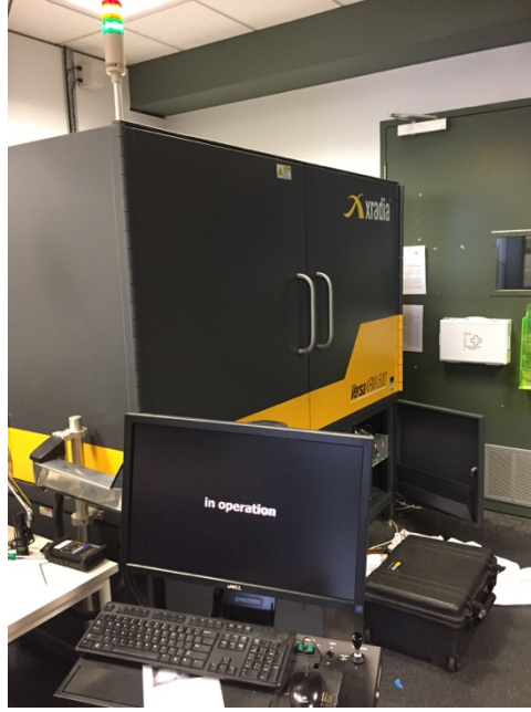
Figure 2.2: X-Radia-Zeiss Versa XRM500 which is used to acquire micro-CT images of the samples.
