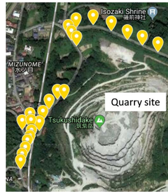
Figure 5. Points of ground vibration measurement.
