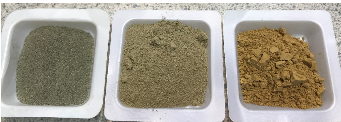
Figure 5-17: DT ore changed in colour from brown at 53 µm (rightmost) to brown-grey at 10 µm (middle) to light grey at 5 µm ( leftmost)
