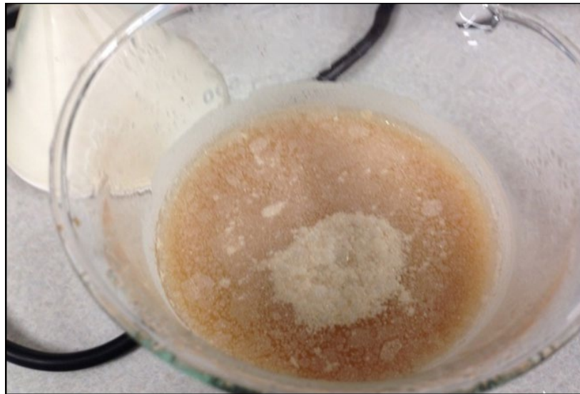
Figure 5-19: Floating calcium sulfates scales observed on prolonged leaching of DT ore (Lim, Ibana et al. 2016)
