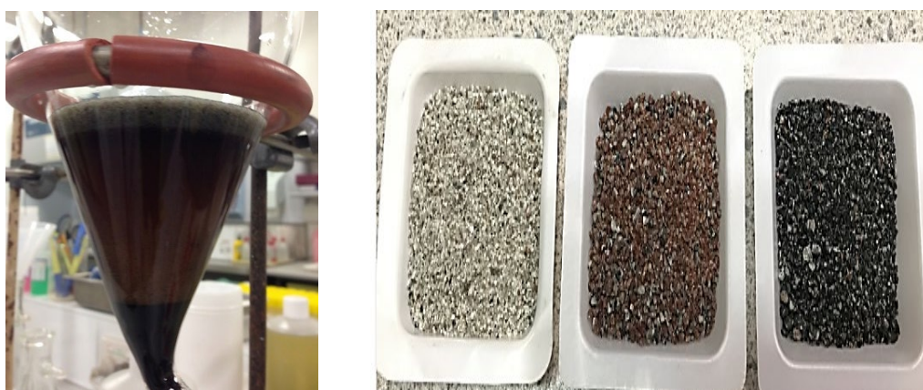
Figure 4-3: Photo images of SG ore beneficiated via heavy media separation (left) and mineral fractions recovered as red eudialyte minerals, black arfvedsonite minerals and white aegirine minerals (right)
