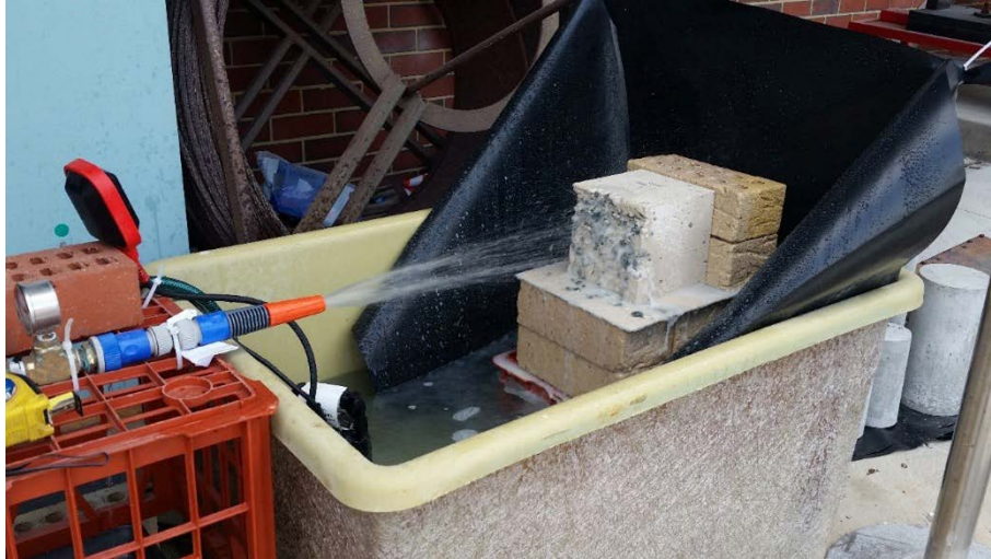
a. Schematic b. Experimental setup Figure 5-9 Accelerated erosion test
