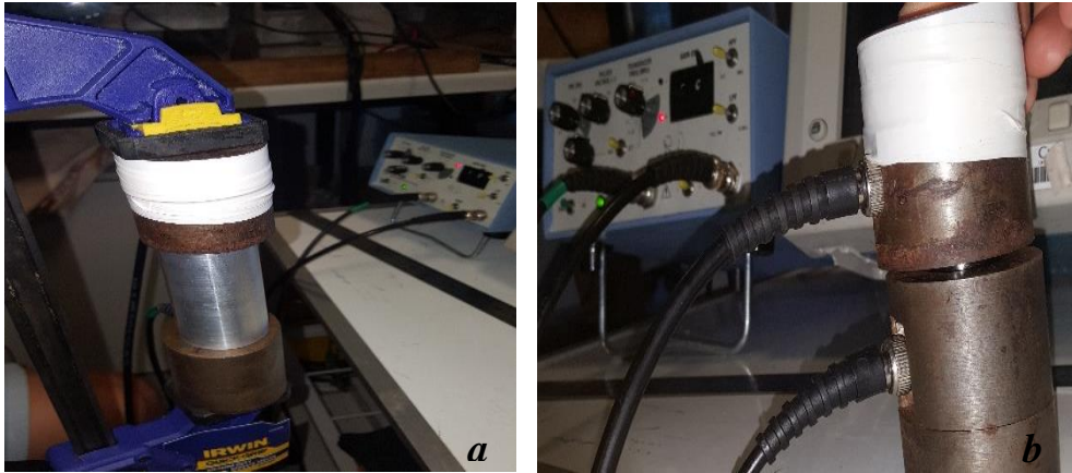
Figure 4.1: A photo of the cylindrical AL sample in contact with S-wave transducers (a). S-wave source and receiver in contact (b).
