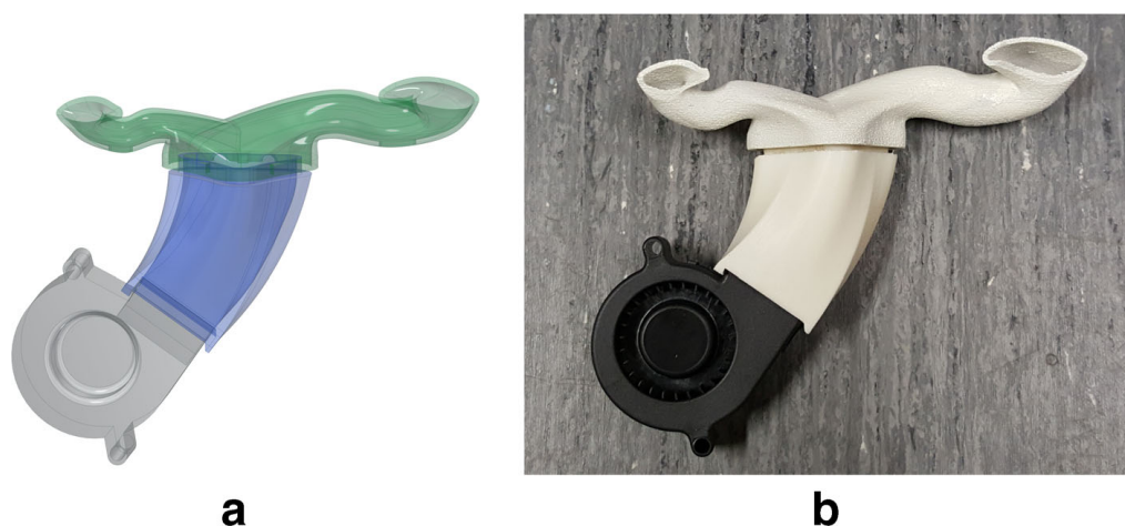
Fig. 7 Lens condensation blower and ducting. a The CAD design showing the complex ducting geometry. b The manufactured ducting assembly removed from the observatory with the blower
