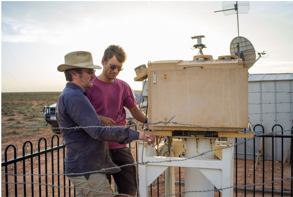
Fig. 2 DFN large format film based observatory — used in initial phase, prototype digital observatory visible in background
