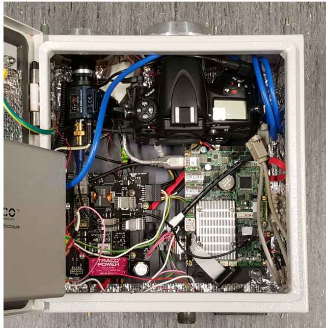
Fig. 6 Fireball observatory internals. Showing (clockwise from top left): video camera and lens, blower ducting, camera and lens (LC shutter inside), embedded PC, observatory management PCB (microcontroller, GNSS module), hard drive enclosure
