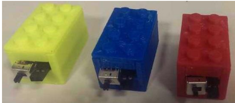
Figure 4.6: First prototype sensor set with Lego shaped cases
