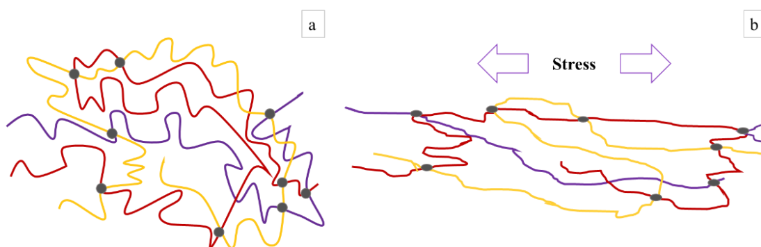
Fig. 2. 1. Reversible extension of cross-linked elastomer chain: (a) undeformed, (b) deformed.
