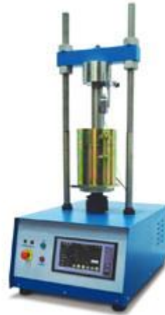
Figure 2.31 A typical CBR testing machine by Cooper technology.
