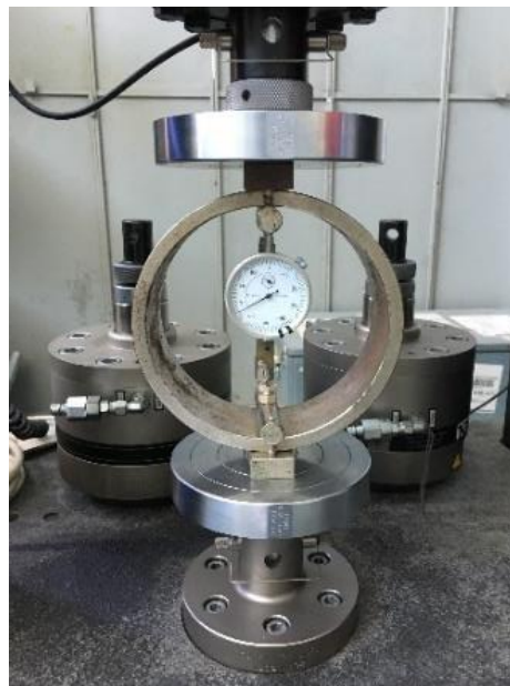
Figure 3.3 Experiment of the conventional proving ring
