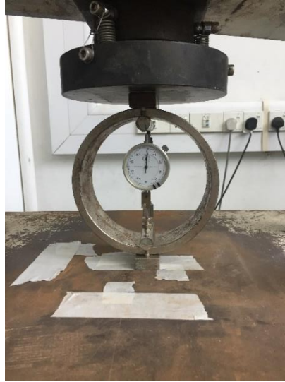
Figure 2.1 A proving ring under axial load
