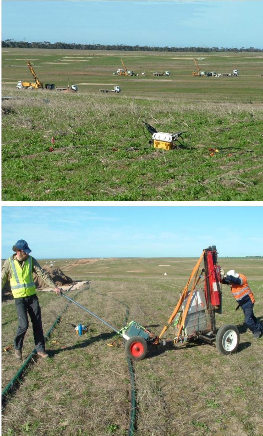
Figure 4.18 Field Equipment used for the 2D seismic survey at the Hillside mine. Distributed seismic array (above panel, 300 ch) and weight drop (below panel).
