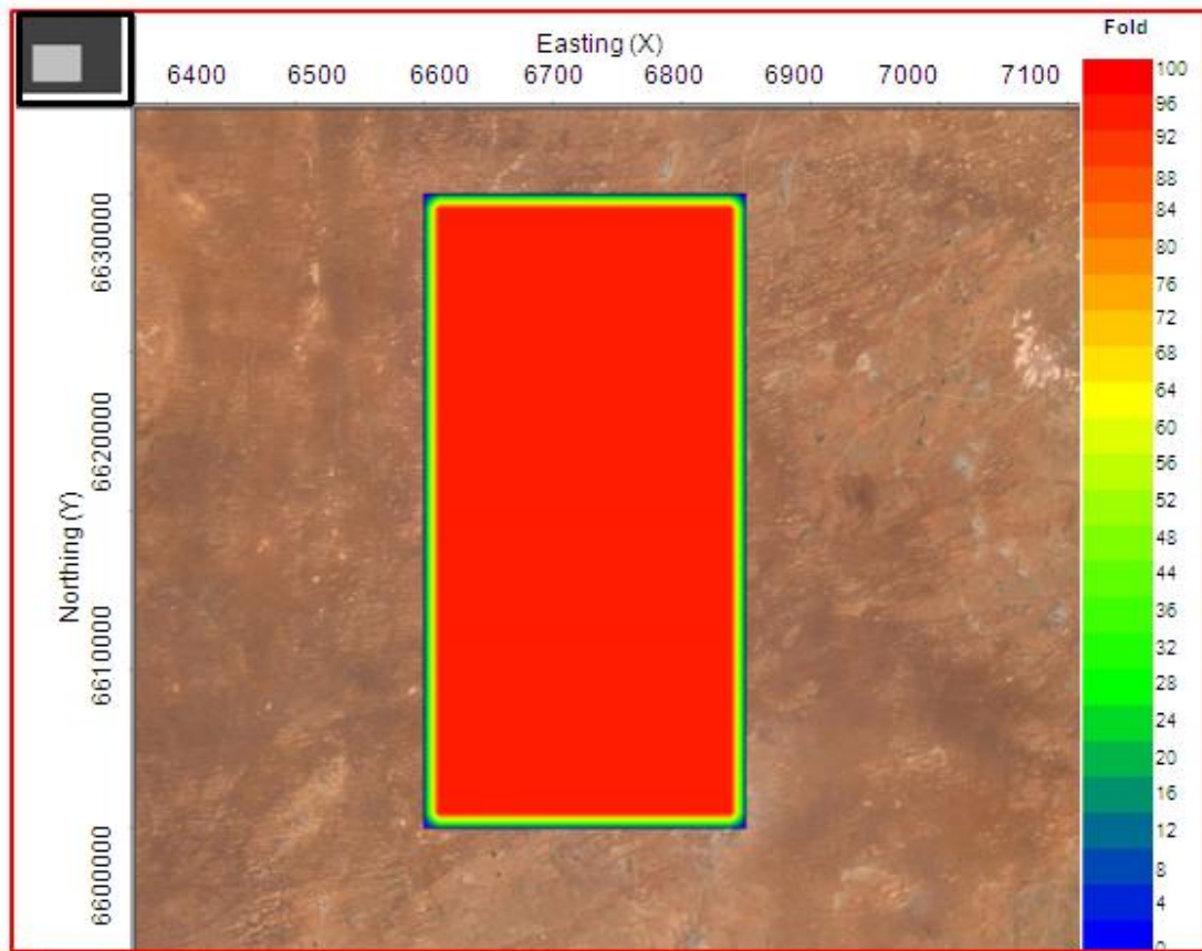
Figure 8.2 The field map at 1500 m depth overlain on a satellite photo of the area around Olympic Dam. Approximately 1000 sq. km of area is covered by the survey that uses an orthogonal design with survey geometries typical of many petroleum exploration surveys.
