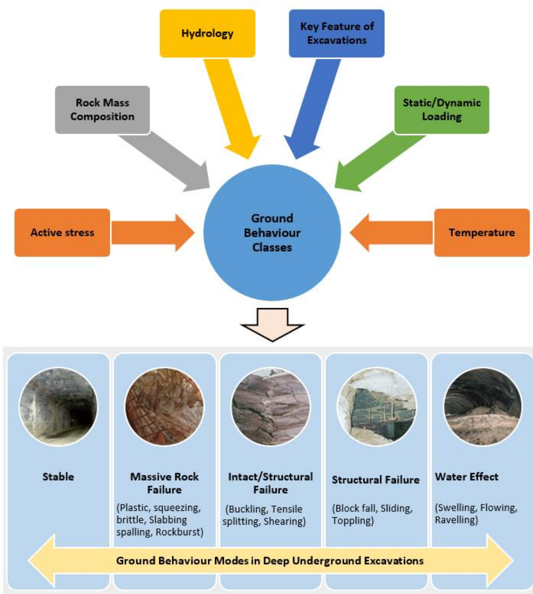
Figure 4.17. Ground behaviour modes in deep underground excavations
