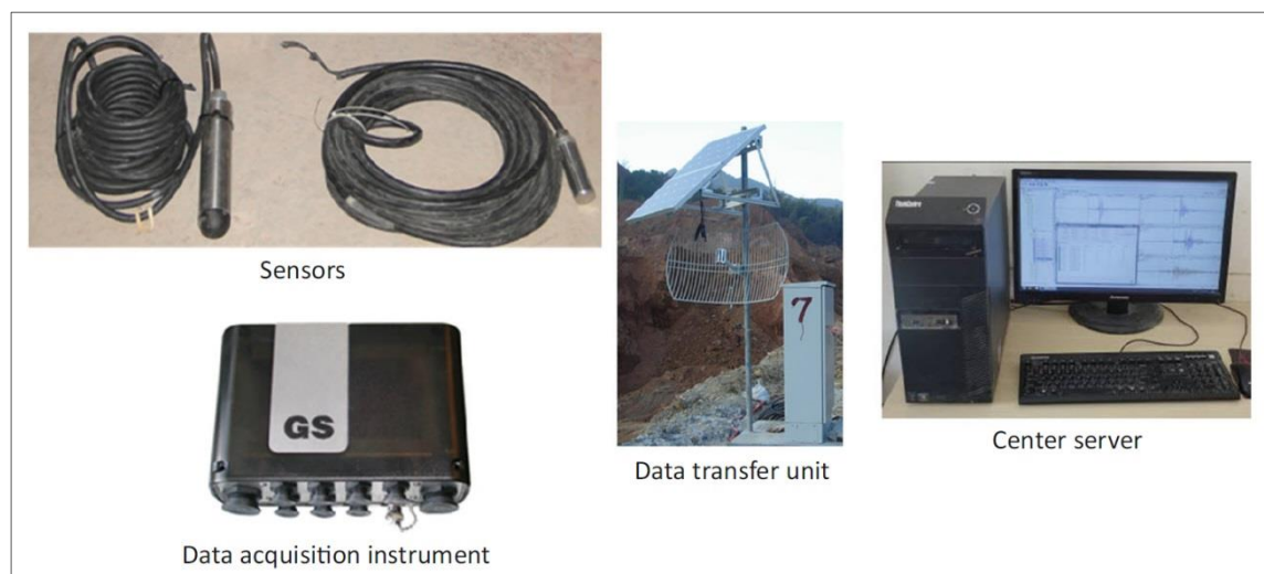
Figure 8.6. The main components of the seismic monitoring system (Xiao et al., 2016)
