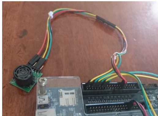
Fig. 4.33: Experimental Set-up of LV-MaxSonar-EZ Sensor
