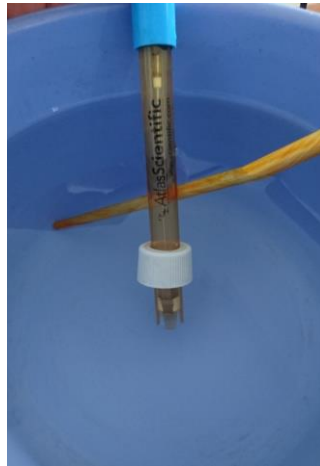
Fig. 5.4: Sensing Area of pH probe immersed in Water
