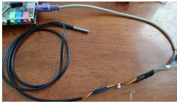
Fig. 4.30: Experimental Set-up of DS18B20 Sensor
