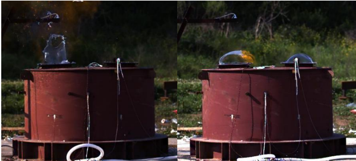
(a) Design case No. 4 with one vent panel (b) Design case No. 5 with two vent panels Fig. 6 9.5 vol % gas concentration experiments for case No.4, No.5
