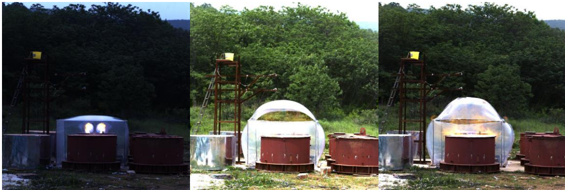
(a) 500mm separation distance (b) 750mm separation distance (c) 1000mm separation distance Fig. 11 Snapshots of different separation distance cases in experiments
