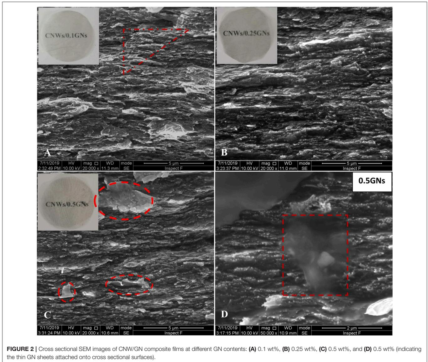
**FIGURE 2** | Cross sectional SEM images of CNW/GN composite films at different GN contents: **(A)** 0.1 wt%, **(B)** 0.25 wt%, **(C)** 0.5 wt%, and **(D)** 0.5 wt% (indicating the thin GN sheets attached onto cross sectional surfaces).
