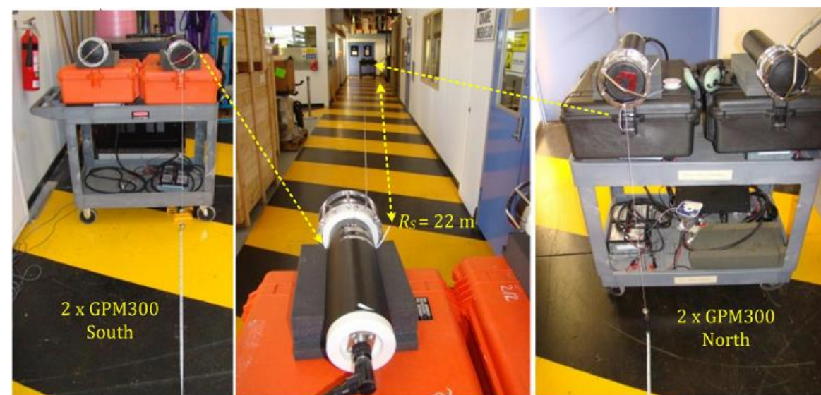
Figure 148 Air testing at 21.47 m range configuration
