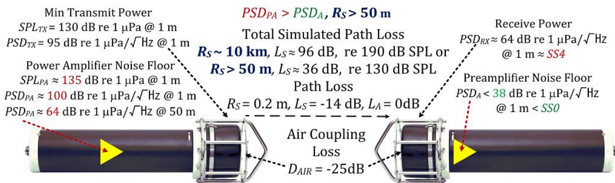
Figure 146 Air 0.2 m range sonar equation diagram
