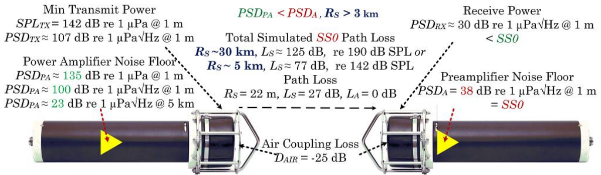
Figure 150 Air 22 m range testing sonar equation diagram
