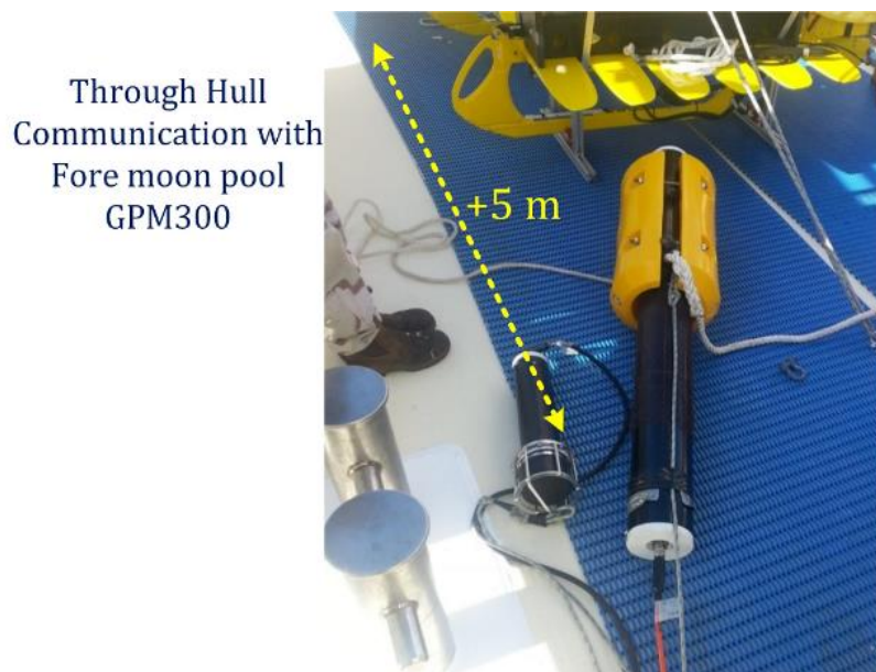
Figure 198 GPM300 through vessel hull super structure communication deck test
