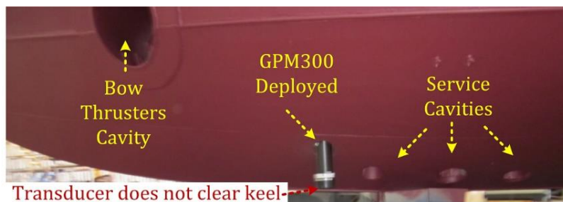
Figure 204 GPM300 deployed through RV Whale Song moon pool
