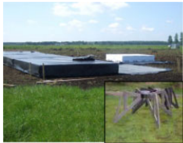
Figure 6b. An example of sparse aperture array technology from the LOFAR telescope (ASTRON): A “tile” of LOFAR high-band antennas, with the individual elements shown in the inset.
