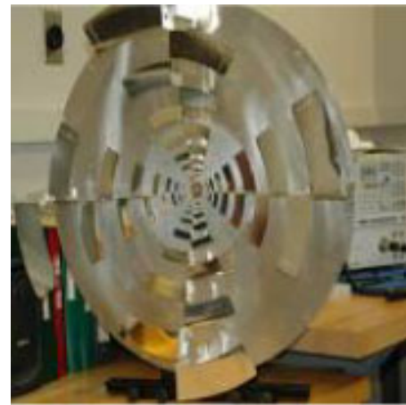
Figure 8d. An example of a new single-pixel, wideband feed for reflector antennas: A quasi self-complementary antenna [13]. All of these dual-polarization feeds shown in Figure 8 are being evaluated for use with the SKA (illustrations courtesy of G. Cortes Medellin).
