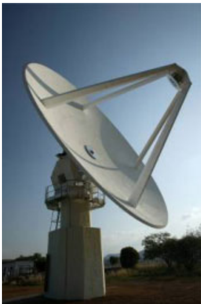
Figure 12a. An experimental dish antenna. The MeerKAT 15 m diameter dish constructed with low-cost fiberglass material and flame-sprayed aluminum reflective layer. The 2 mm rms surface accuracy allows effective operation to about 10 GHz. This is a platform designed to test various design concepts, but is unlikely to be the actual design used in SKA Pathfinders
