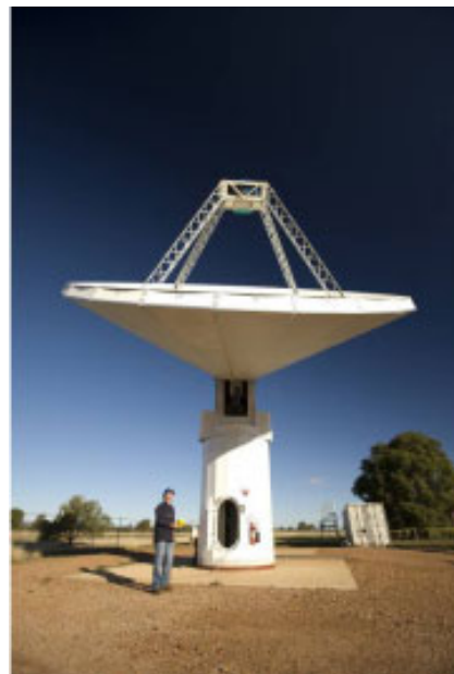
Figure 12b. An experimental dish antenna. The ASKAP 12 m test antenna at Parkes. The Chequer Board feed shown in Figure 10a is mounted at the prime focus of the dish. The antenna uses a stretch-formed panel construction and operates to beyond 20 GHz; it is supplied by Patriot Antenna Systems, Inc. This is a platform designed to test various design concepts, but is unlikely to be the actual design used in SKA Pathfinders.
