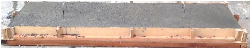
Figure 4.7: Freshly casted concrete wall specimen
