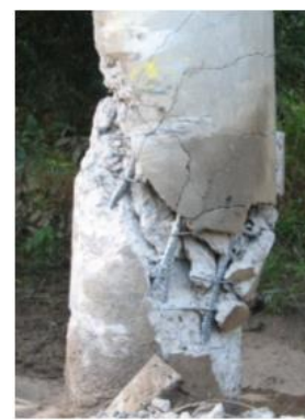
(a) Flexural cracks (b) Shear failure at the column top (c) Shear failure at the impact point
