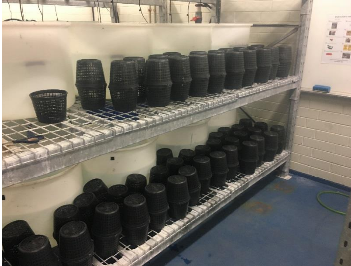
Plate 6.1: The cylindrical white tanks and black planter-basket cages used in the experiment (Cages remained horizontal during the experiment).
