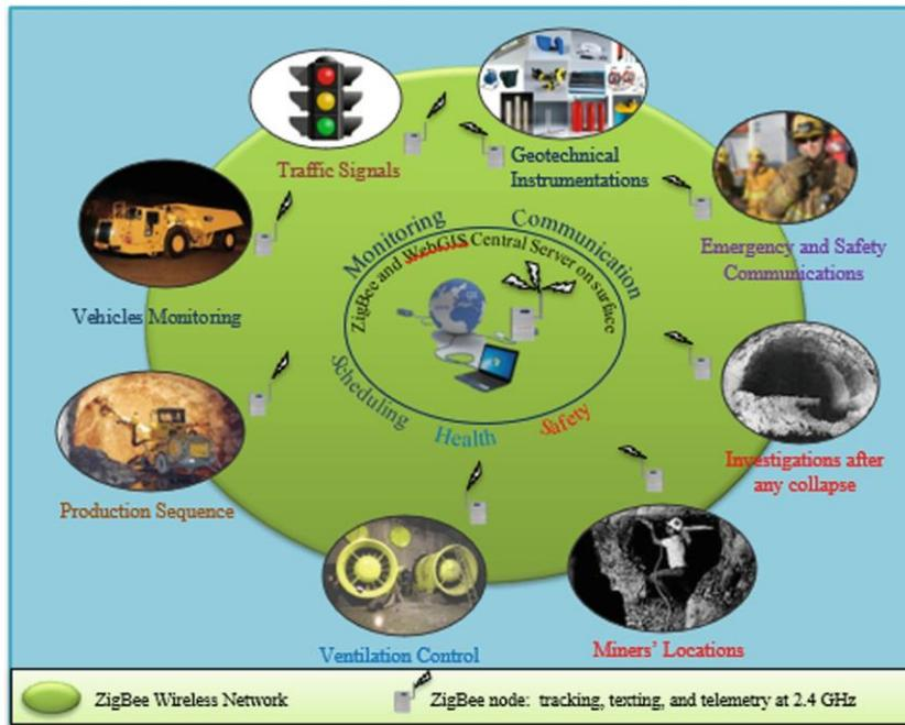
Fig. 2. Applications of WSNs for underground communication and monitoring
