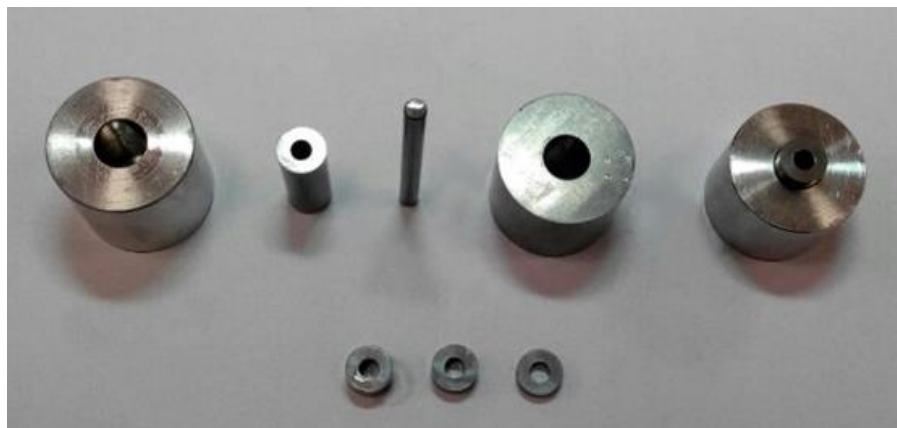
Figure 56. Mold for small coal briquette specimens
