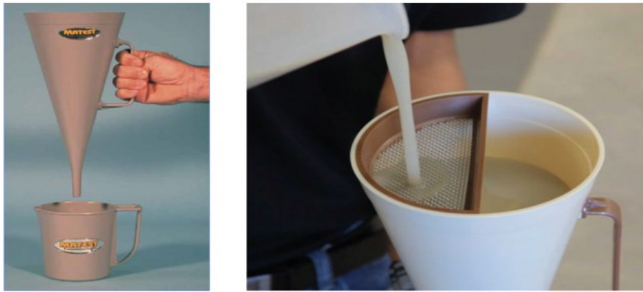
Figure 5: Marsh Funnel viscosity measurement.
