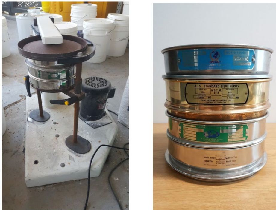
Figure 39: Sieve shaker (left) and sieve meshes (right) for 200 µm, 150 µm, 106 µm, and 75 µm (top to bottom).
