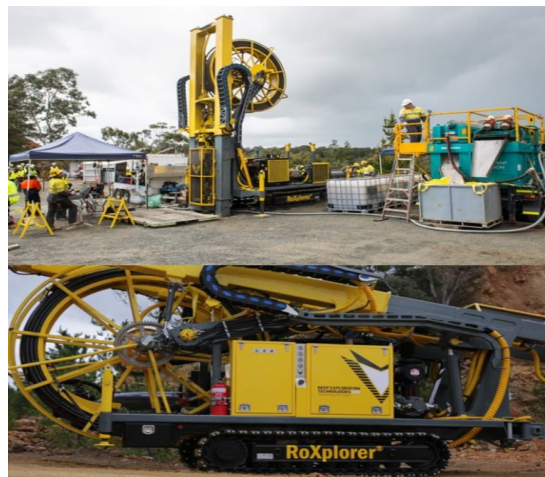
Figure 57: Coiled tube drilling system, RoXplorer, used in the drilling trials in Australia - courtesy DET CRC.
