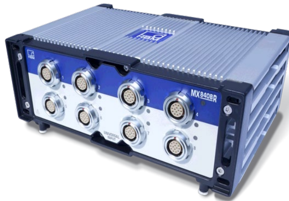
Figure 31: DAQ SomatXR MX840B-R data acquisition system.
