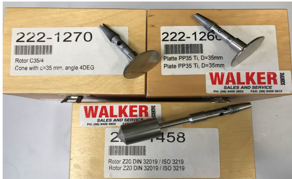
Figure 41: Haake Mars Z20DIN, PP35Ti and C35/4Ti sensor systems.
