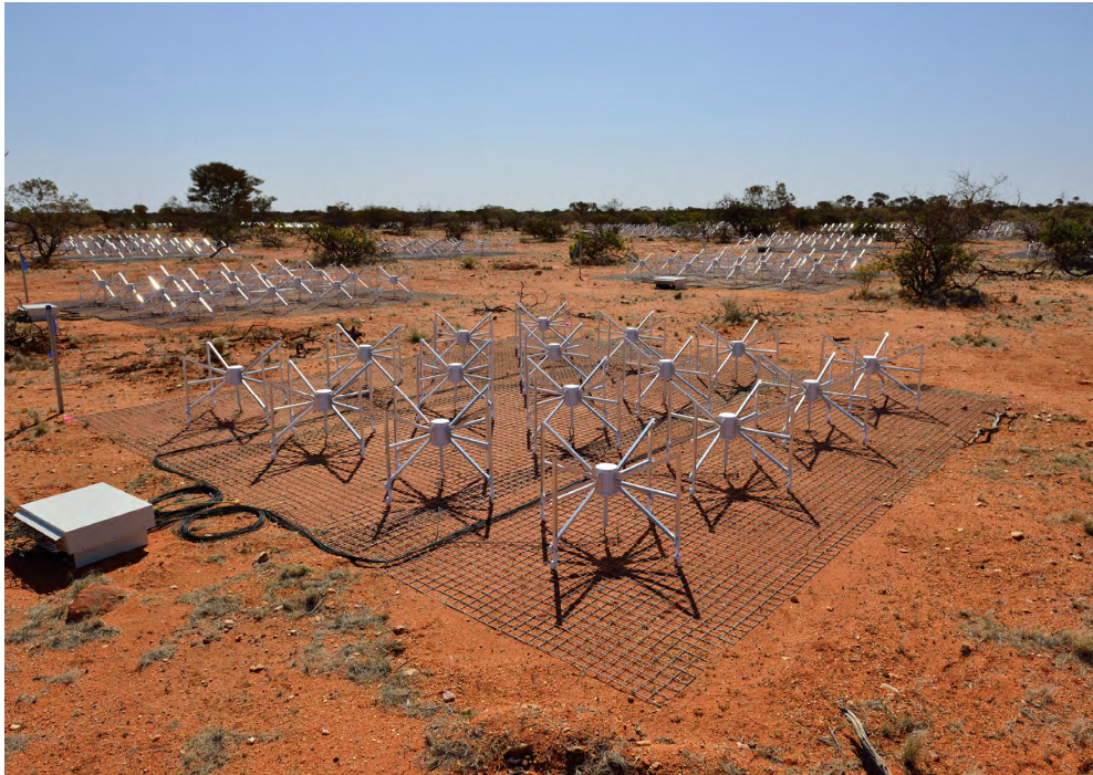
Figure 1.2: An MWA tile connected to a beamformer (white rectangular box). Each antenna element contains a low-noise amplifier (LNA) in the central hub (white cylindrical container). Photo credits: Curtin University and MWA collaboration.
