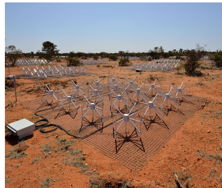
Figure 1. An MWA tile connected to a beamformer (white rectangular box). Each antenna element contains an LNA in the central hub (white cylindrical container). Photo credits: Curtin University and MWA Collaboration.
