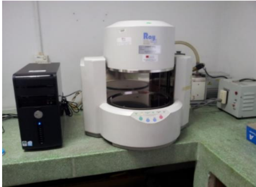
Figure 3. 6: XRF machine for chemical composition of the POFA.
