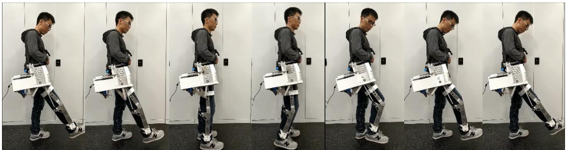
Fig. 4.13 Gait cycle of the leg exoskeleton
