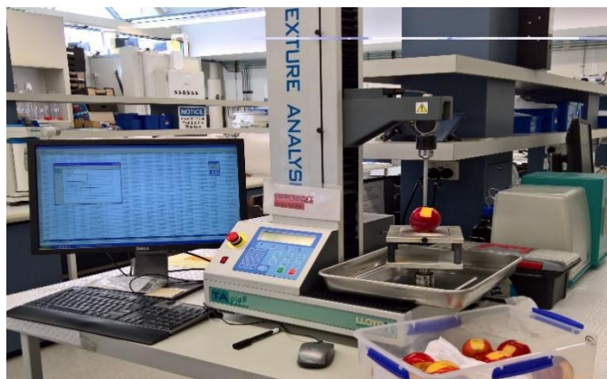
Fig. 3. 11 Testing the fruit firmness of ‘Diamond Bright’ nectarines by using Texture Analyser (TPA Plus, AMETEK Lloyd Instruments).
